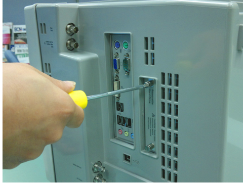
Figure 3-9 Unscrew the hard drive
