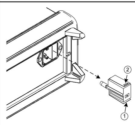
**2** Remove the line voltage selector from fuse holder assembly.
