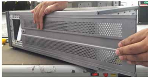
L4491A Install Side Cover (Option STD and Option 001)
