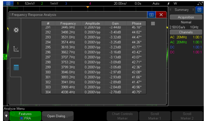
Figure 5. Exportable (.csv format) gain and phase numerical test results of a series R-L-C bandpass filter.
