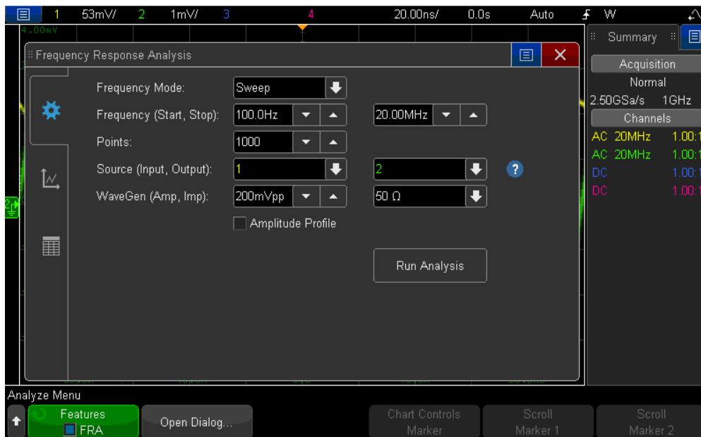
Figure 3. InfiniiVision “Settings” menu used to establish test conditions for a frequency response analysis test.
