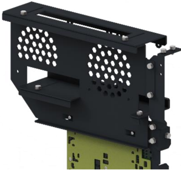
Figure 3. PCIe Card Holder provides mechanical stability.
