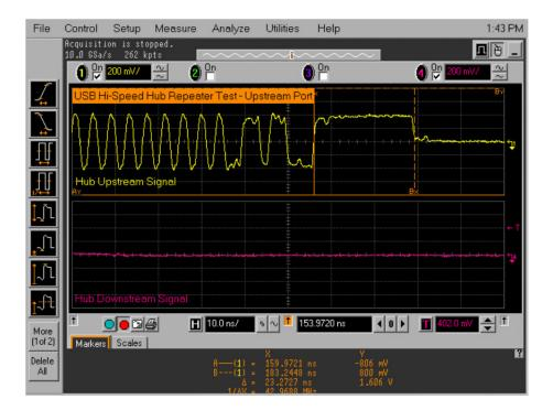
Verify also that the EOP in Channel 4 is not corrupted.
