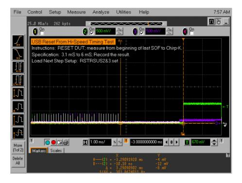
The device should transmit a CHIRP handshake following the reset.
