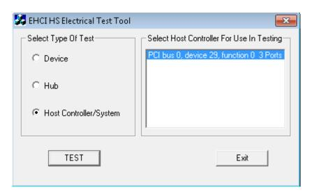
3 The Host Test menu of the HS Electrical Test Tool should appear as below.
