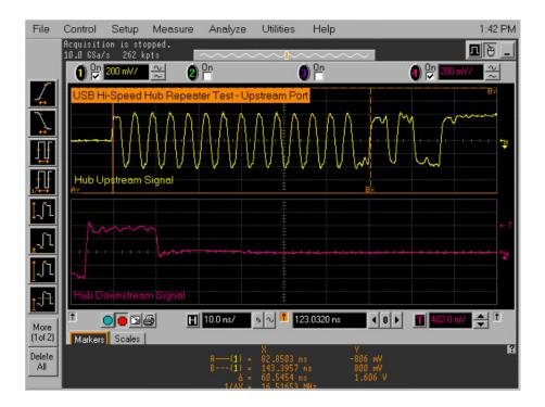
Measure the time of the EOP width of the packet in Channel 1.
