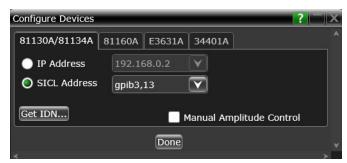
8 Press the "Get IDN" button to verify the connection status. You should see the message box below if successfully connected.
