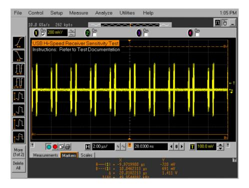
Generates "IN" packets (of compliant amplitude) with a 32-bit SYNC field as shown below.
