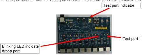
11 To exit manual mode, press S2 and while holding it down, press S1. All of the LEDs will go off.
