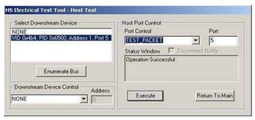
2 Using the oscillopscope, verify SOFs (Start of Frame packets) are being transmitted by the port under test. You may need to lower the trigger level to somewhat below 400 mV to obtain a trigger.
