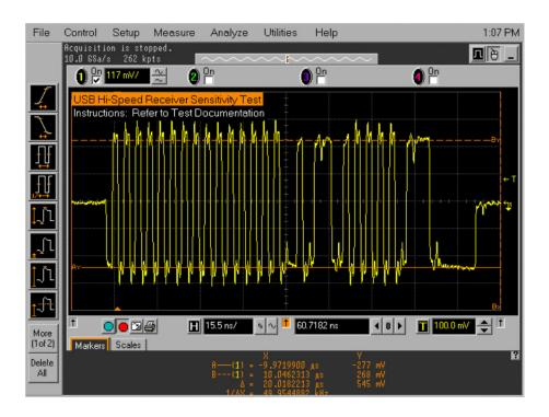
Using the oscilloscope markers, measure the packet amplitude
