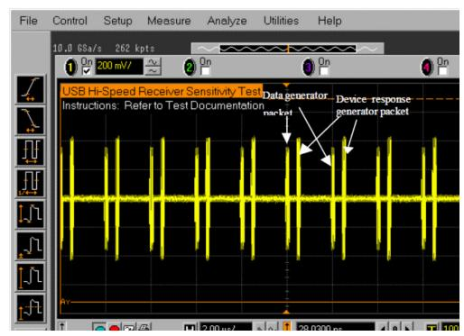
Reduce the amplitude of the data generator packets in 20 mV steps (on the generator before the attenuator) while monitoring the NAK response from the device on the oscilloscope.
