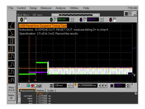
The device responds to the reset with the CHIRP-K.
