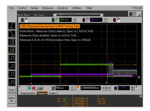
Using the markers, measure the time from the beginning of the last J in the CHIRP K-J-K-J (3 pairs of CHIRP-K-J's) to the time when the device turns on the Hi-Speed terminations, as shown in the following figure.
