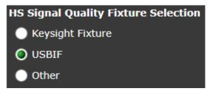
These settings affect ONLY the HS Signal Quality tests. They can be used to embed/de-embed the fixture. These settings DO NOT remove the differential probe or SMA cables.
