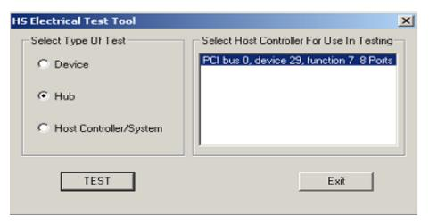
2 The hub under test should be enumerated with the hub's VID shown together with the USB address. Select [TEST\_PACKET] from the Hub Command drop down menu and click [EXECUTE].
