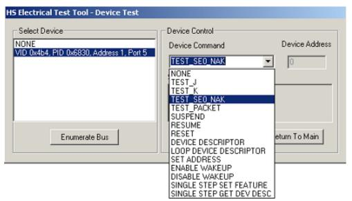
3 Place the test fixture Test Switch (S1) into the **TEST** position. This switches in the data generator in place of the host controller. The data generator emulates the "IN" packets from the host controller.
