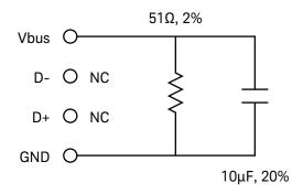
Figure 8 100 mA Load Board Schematic
