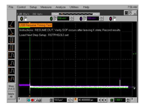
The device should resume the HS operation, which is indicated by the presence of HS SOF packets (with 400 mV nominal amplitudes) following the K state driven by the host controller, as shown in the previous figure.
