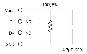
Figure 9 500 mA Load Board Schematic
