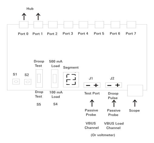
Connecting the Equipment (if you do not have the new E2649-66405 Droop/Drop Test Fixture)
