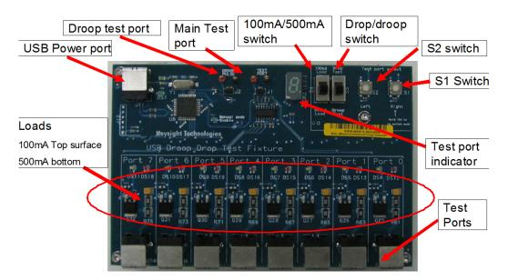
To begin, plug the USB cable from your oscilloscope into the USB Power port to power the test fixture. The DS1 LED should illuminate (green LED). See the picture below for the location of DS1 (the picture is zoomed in on the upper left hand corner of the test fixture).
