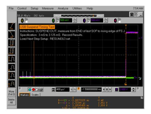
Using the oscilloscope markers, measure the time interval from the end of last SOF packet issued by the host to when the device attached its full speed pull-up resistor on D+, as shown in the previous figure.
