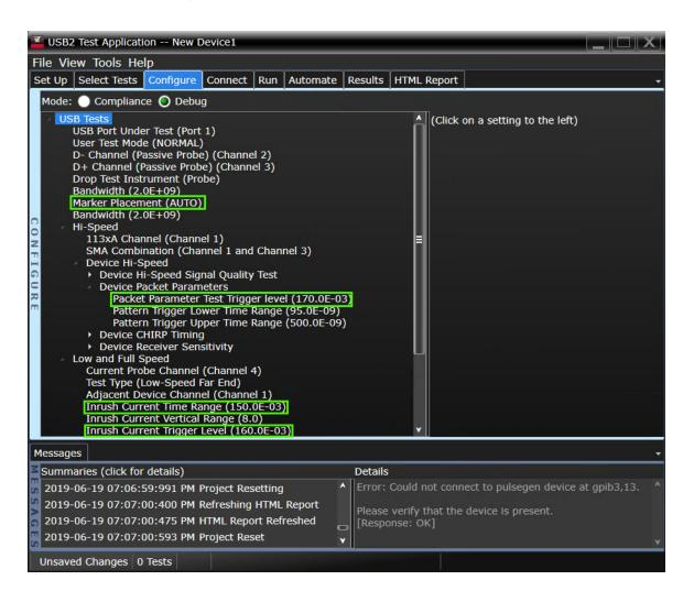
Figure 7 Debug Mode Options for Hi-Speed Testing
