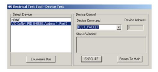
3 Place the Test Switch (S1) in the **TEST** position. Verify the yellow TEST LED is lit. You should see the transmitted test packet on the oscilloscope as below.
