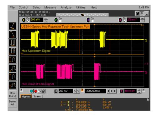
Count the number of bits in the sync field on the third packet in Channel 1.
