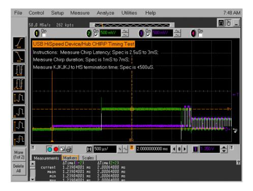
Figure 10 Measure the device's CHIRP-K latency in response to the reset from the host port
