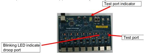
11 To exit manual mode, press S2 and while holding it down, press S1. All of the LEDs will go off.
