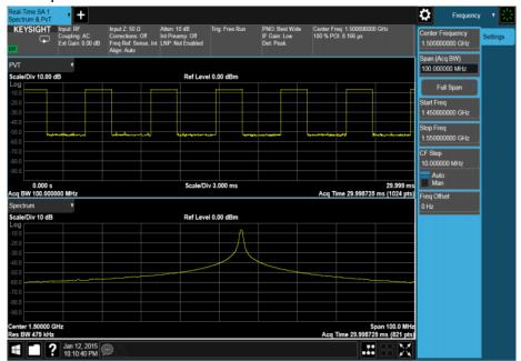
The PvT Spectrum provides a dual view with the top window showing the Power vs Time trace and the bottom window showing the Spectrum trace.
