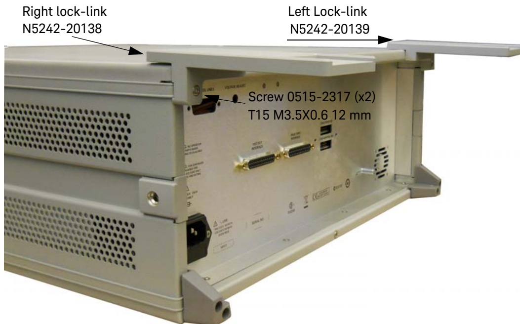
Figure 7 Install Lock-links to the Test Set
