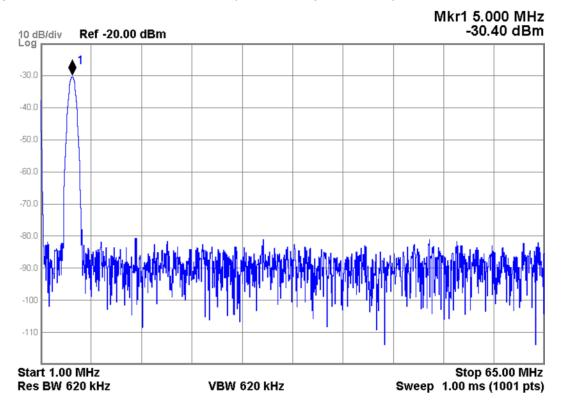
**10.**Vary the frequency of the Direct Digital Synthesizer alignment signal across its frequency range and verify that the signal level remains greater than –35 dBm up to 40 MHz. Above 40 MHz the signal level should remain greater than –40 dBm.
