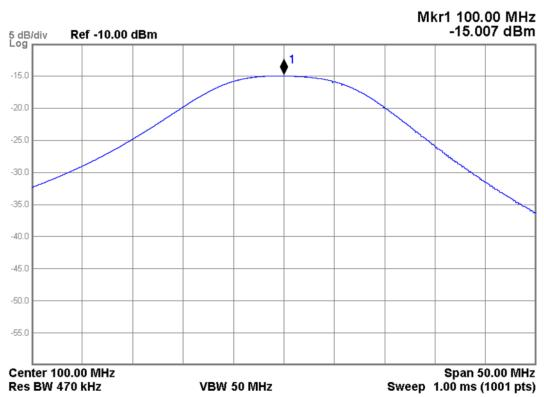
Figure 5-24 A22 Radiated Filter Assembly - Band 2 Filter Path
