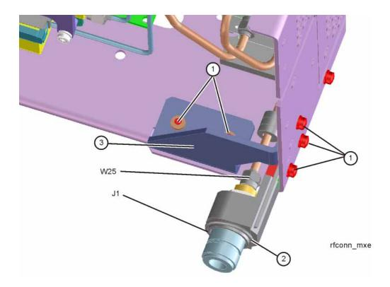
**4.** Remove the two screws **(1)** (0515-0372) that attach the Input Connector Assembly to the chassis. The connector assembly can now be lifted from the chassis.
