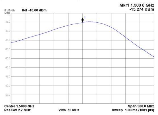
Figure 5-28 A22 Radiated Filter Assembly - Band 6 Filter Path
