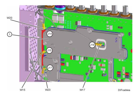
**4.** Refer to Figure 18-54. Pull the AIF/DIF assembly part way out of the chassis. Remove cables W16, W17, and W19 from the AIF assembly.
