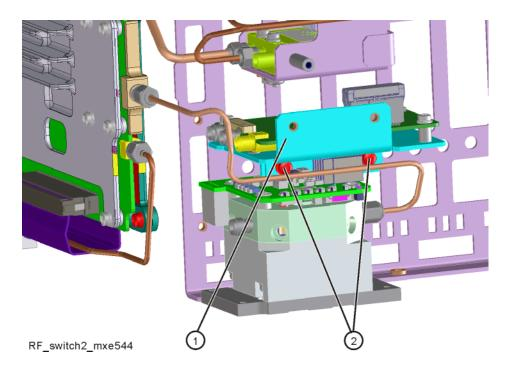
Figure 18-28 RF Switch/High Band Preamp Assembly and Bracket Separation - Option 544
