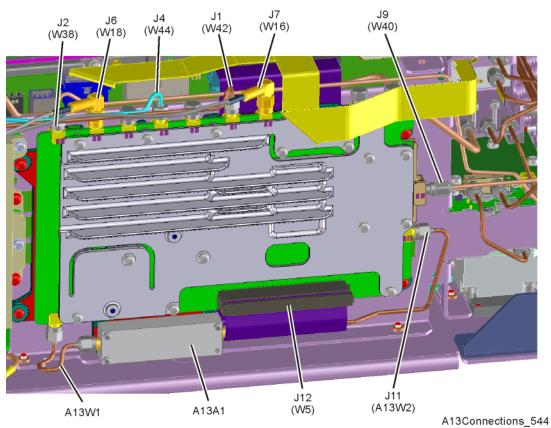
Figure 6-18 A13 RF Front End Assembly Connections - Option 544
