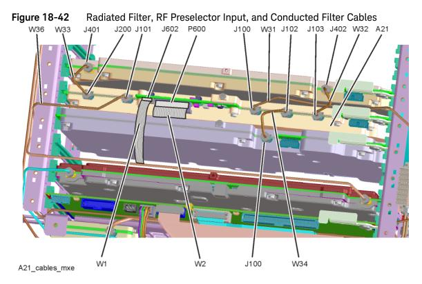
**5.** The Radiated Filter assembly can now be unplugged from the motherboard by using the ejector on the Radiated Filter assembly to disconnect from the motherboard and lift out of the chassis.
