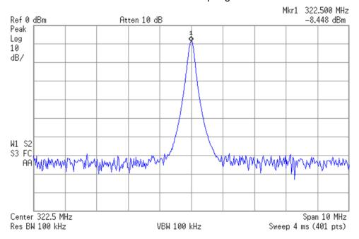
**3.** If the signal level is incorrect the most likely cause of the problem is the A13 RF Front End assembly itself.
