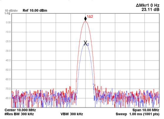
**14.**Turn the instrument Preamp off by pressing **AMPTD**, **More**, **Internal Preamp**, **Off**.
