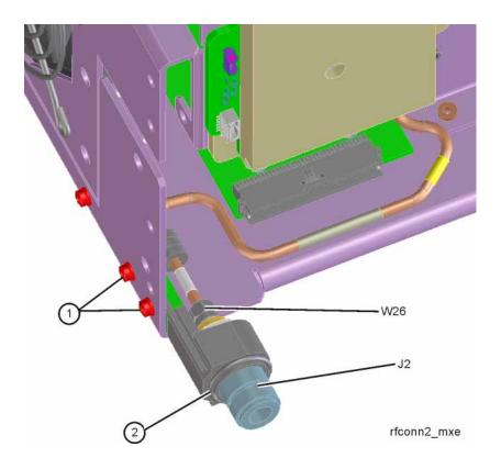
**4.** Remove the two screws **(1)** (0515-0372) that attach the Input Connector Assembly to the chassis. The connector assembly can now be lifted from the chassis.
