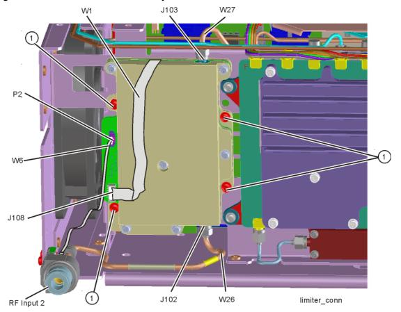
Figure 4-16 A23 Limiter Assembly Connections
