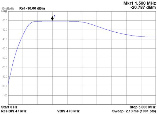
Figure 5-34 A24 Conducted Filter Assembly - Band 4 Filter Path
