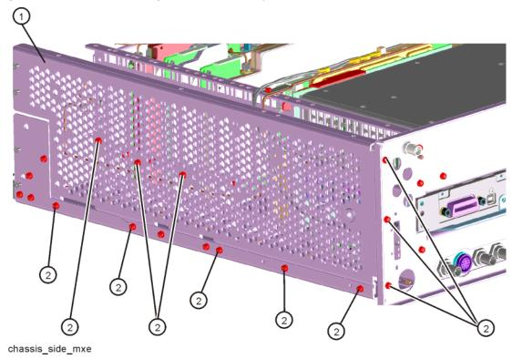
Figure 18-7 Chassis Right Side Outer - Option 503, 508, & 526
