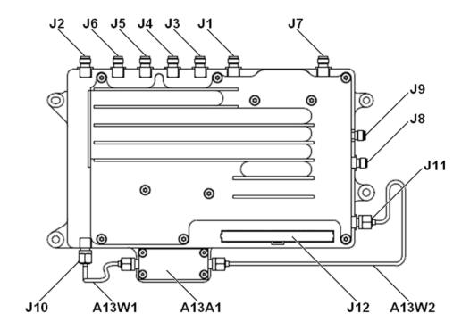
Figure 18-36 RF Front End Assembly Cable Removal - Option 544
