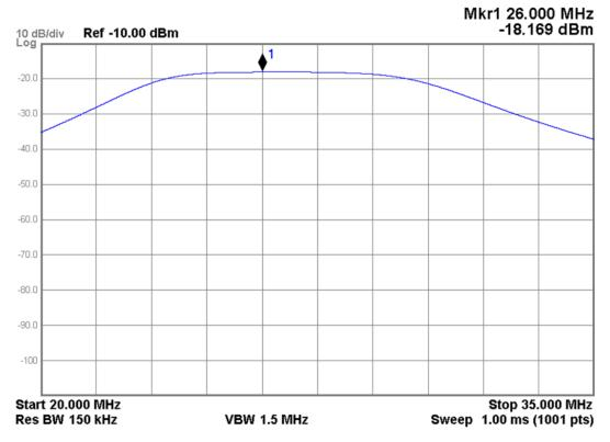
Figure 5-42 A24 Conducted Filter Assembly - Band 12 Filter Path
