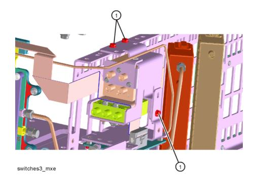
**3.** Refer to Figure 18-20. Replace cables W27, W30, and W31. Torque to 10 inch-lbs.
