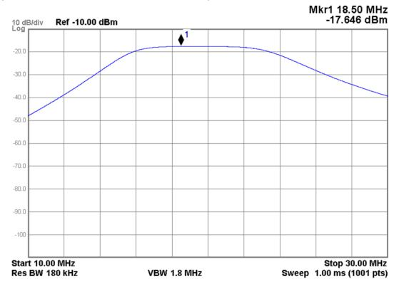
Figure 5-40 A24 Conducted Filter Assembly - Band 10 Filter Path
