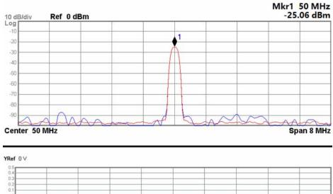
8. If the signal level measured is correct the overall basic functionality of the A25 Wideband Analog IF assembly is working as it should. If not, proceed with the rest of the verification listed in this section.
