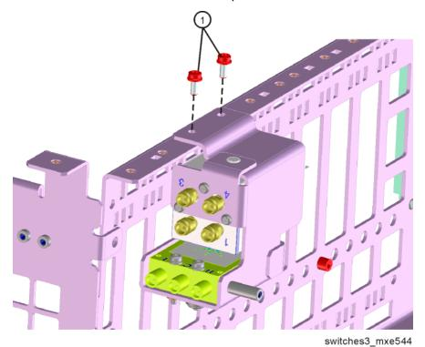
**3.** To separate the Cal Switch (1) from the bracket (5) (N9020-80057), remove the two screws (2) (0515-1410).
