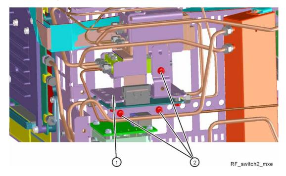
Figure 18-11 RF Switch/High Band Preamp Assembly and Bracket Separation - Option 503, 508, & 526
