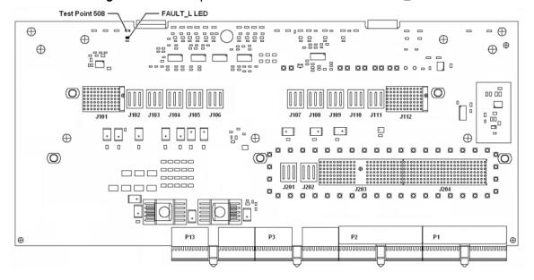
Figure 2-6 A7 Midplane Board - Test Point 508/FAULT\_L LED
