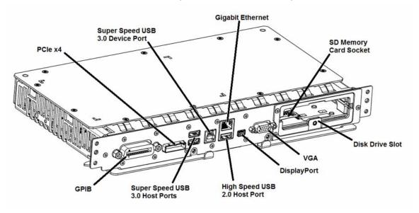
CPU & Disk Drive A4 Processor Assembly Description
