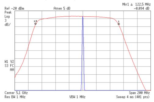
i. Verify that the A13A1 Bandpass Filter insertion loss at 5.1 GHz is approximately 2 dB, allowing for any additional test cable loss, and the 3 dB bandwidth is at least 100 MHz, as shown in Figure 6-20.
