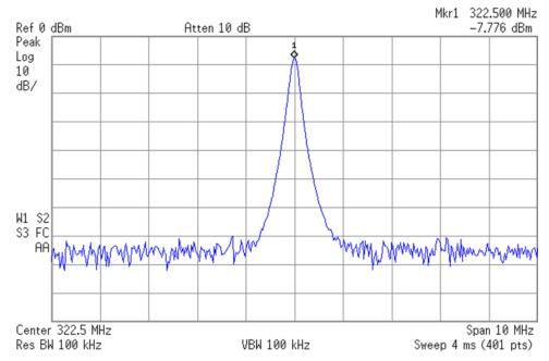
**13.**If the signal level is incorrect the most likely cause of the problem is the A13 RF Front End assembly itself.
