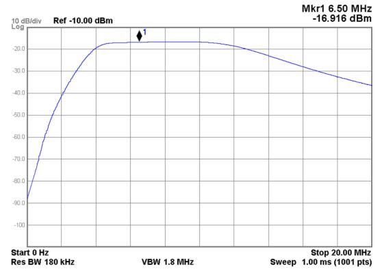
Figure 5-36 A24 Conducted Filter Assembly - Band 6 Filter Path
