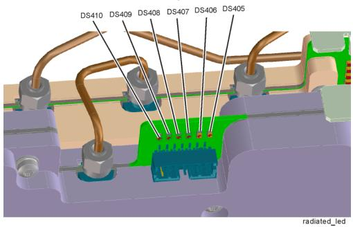
Table 5-7 A22 Radiated Filter Assembly Status LEDs
