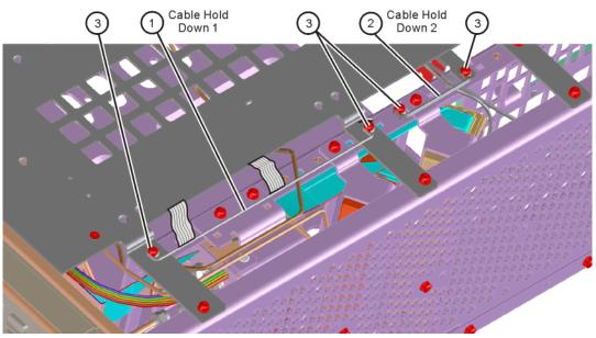
1. Refer to Figure 18-4. To replace the top brace or the power supply bracket, place them into the correct position and attach the screws referred to in the removal process. Reinstall wire hold down 1. Torque to 9 inch-pounds.
