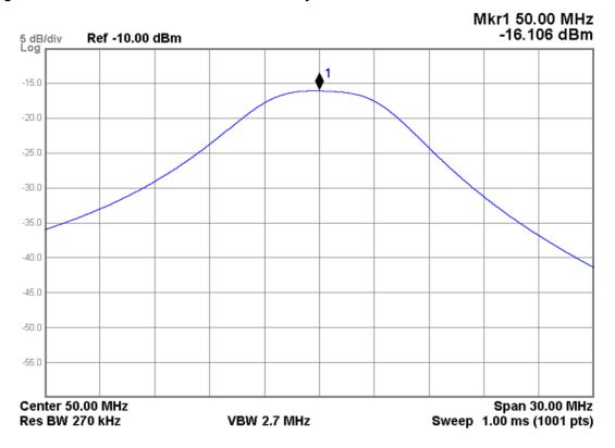
Figure 5-23 A22 Radiated Filter Assembly - Band 1 Filter Path
