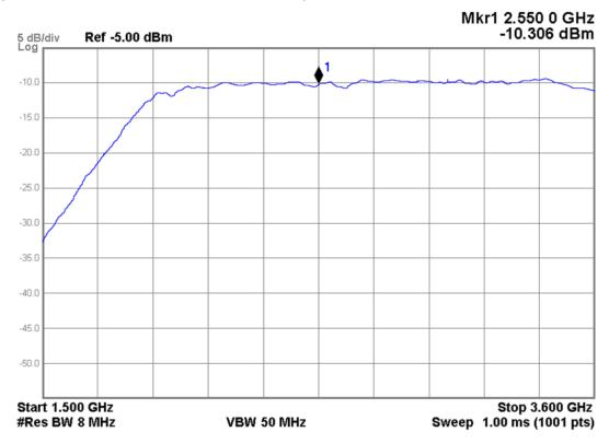
Figure 5-29 A22 Radiated Filter Assembly - Band 2 Through Path
