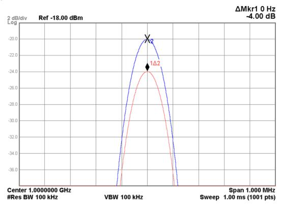
Figure 4-9 A9 Attenuator A –4 dB
