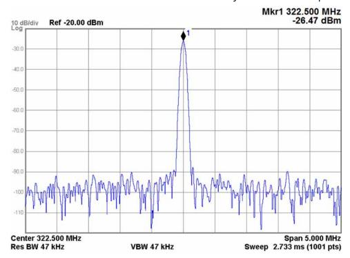
11.If the level is not correct, measure the input signal level coming to A15 J902 out of W14, as shown in Figure 8-6. It should be at approximately the same level shown in Figure 8-14.
