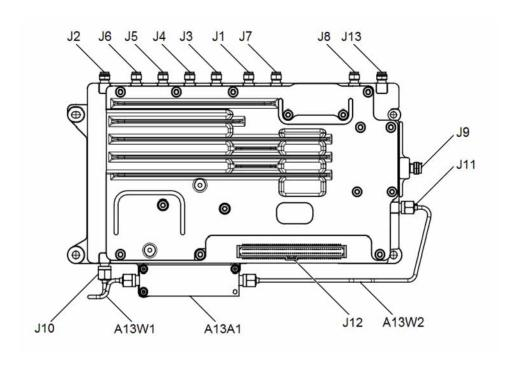
**6.** Remove the 50  $\Omega$  terminators from RF Front End Assembly.
