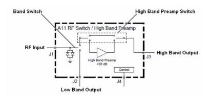
Figure 8-10 A11 RF Switch / High Band Preamp Control Front End Test Board
