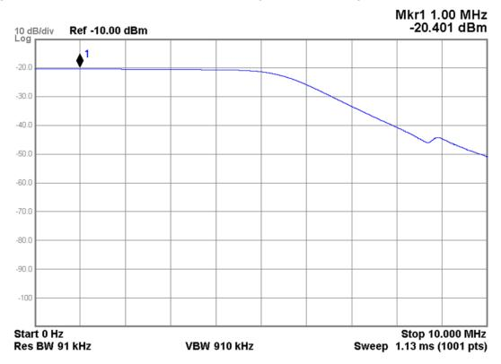
Figure 5-44 A24 Conducted Filter Assembly - Band 1 Through Path
