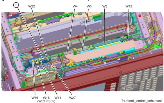
3. Connect the A9 / A10 Input Attenuator Control cable from J801 to the Front End Control Test board J3 & J4 as shown in Figure 8-3.
