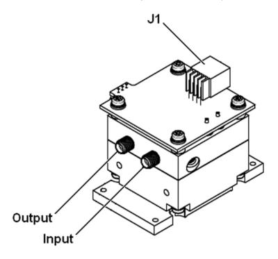
Figure 6-4 A12 YTF Preselector Assembly Connections - Option 544
