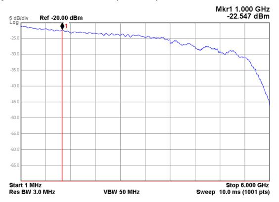
Pre-Filter Shape Verification - Radiated Band
