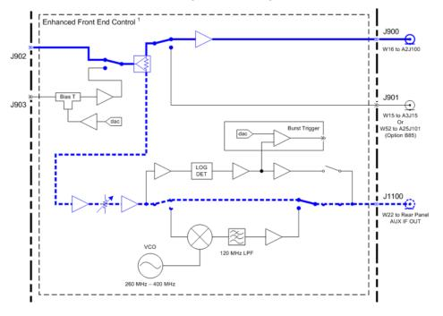
The following procedure will verify the 322.5 MHz IF output switching:
