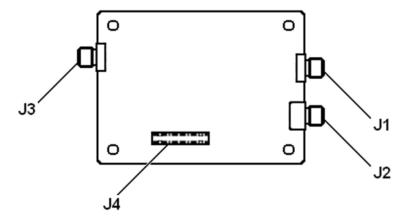
Figure 6-2 A11 RF Switch / High Band Preamp Assembly Connections - Option 544
