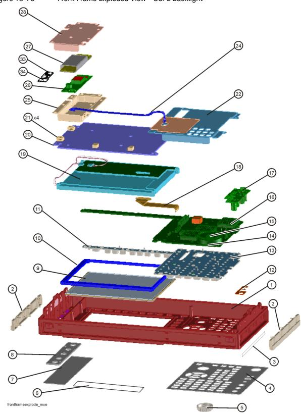
Figure 18-78 Front Frame Exploded View - CCFL Backlight
