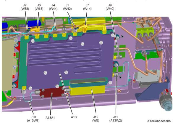
Figure 6-17 A13 RF Front End Assembly Connections - Option 503, 508, & 526
