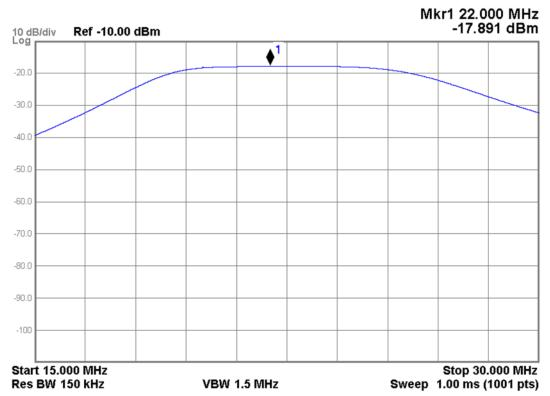
Figure 5-41 A24 Conducted Filter Assembly - Band 11 Filter Path
