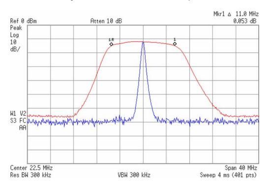
Figure 10-6 A2 Analog IF 1 MHz Filter Path Passband Shape
