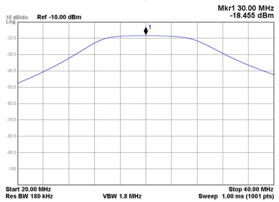
Figure 5-43 A24 Conducted Filter Assembly - Band 0 Through Path
