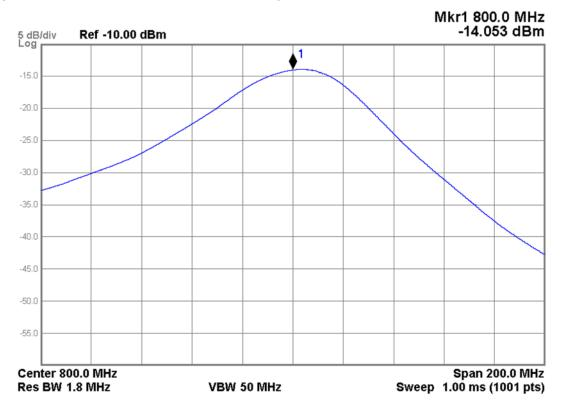
Figure 5-27 A22 Radiated Filter Assembly - Band 5 Filter Path
