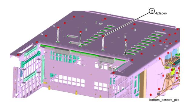
21.Refer to Figure 18-58. Remove the left side chassis (1) (same side as the fan) by removing the nine screws (2) (0515-0372) (six on the bottom).
