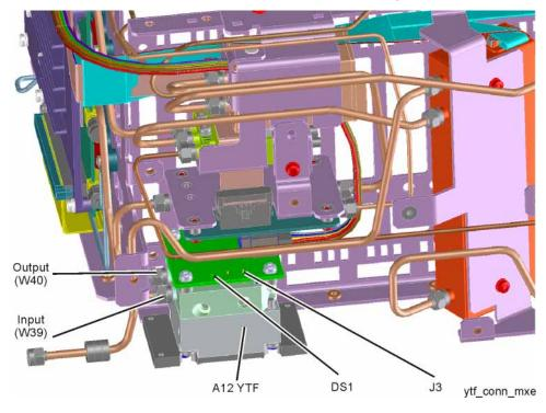
Figure 6-14 A12 YTF Preselector Connector Locations - Option 544
