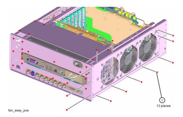
**5.** Refer to Figure 18-63. Unplug the fan wires from the motherboard. The fan assembly can now be lifted from the chassis.
