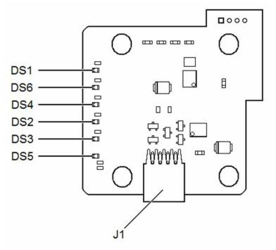
When the instrument is first turned on the only LEDs that should be on are DS1 and DS2. DS1 should be on whenever the instrument is turned on; as this indicates that the voltage regulator on the YTF is working. DS2 will remain on until the assembly has been initialized, which occurs during the time the instrument application initializes the hardware. After that, DS2 will turn off and DS3 will turn on. At the same time that DS3 turns on DS5 will start to blink. It
