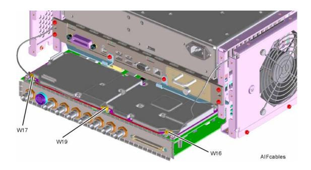
**5.** The AIF/DIF assembly can be removed from the chassis by pulling straight out the back.
