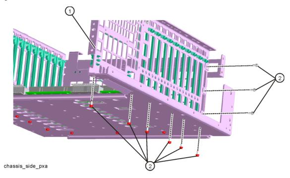
22.Refer to Figure 18-59. Remove the motherboard (1) by removing the four screws (2) (0515-0372). Slide the motherboard back off the standoffs and lift it up and out.
