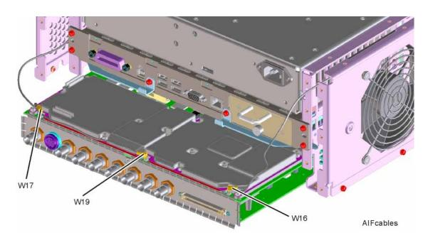
Figure 17-15 AIF/DIF Cables, bottom
