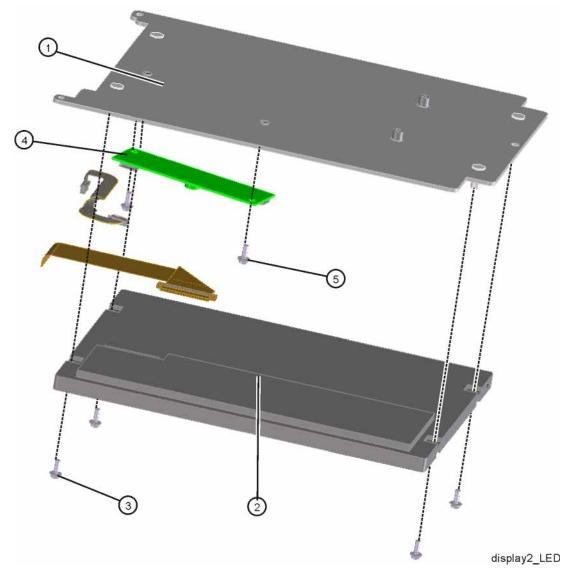
Figure 18-75 LED and Display Bracket Separation
