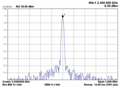
7. If the signal level measured is correct the reference input signal going to the A25 Wideband Analog IF assembly is of the correct level. If not, refer to Chapter 9, "Reference Assembly" and determine why the signal level coming from it is not correct
