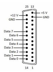
With the use of a voltmeter along with the service menu the operation of each of the individual data lines to the rear panel connector as well as the supply voltages can be verified.
