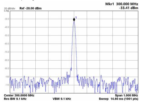
**6.** If the signal level measured is correct the input signal going to the A25 Wideband Analog IF assembly is of the correct level. If not, refer to Chapter 8, "Front End Control" and determine why the signal level coming from it is not correct.
