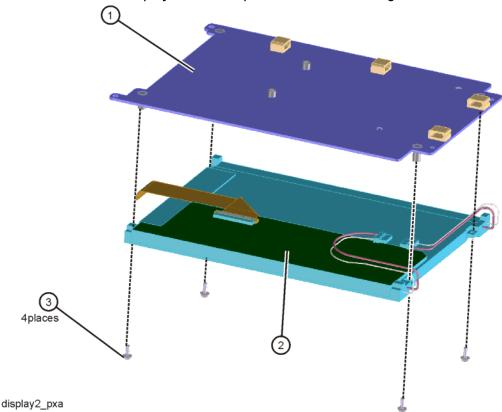
Figure 18-82 LCD and Display Bracket Separation - CCFL Backlight
