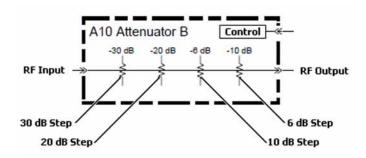
Figure 8-8 A10 Input Attenuator B Control Front End Test Board LEDs
