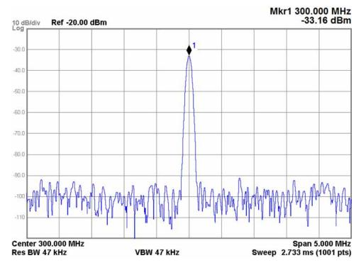
**14.**If the level is not correct, measure the input signal level coming to A15 J902 out of W14, as shown in Figure 8-6. It should be approximately 6 dB higher than the level shown in Figure 8-16.
