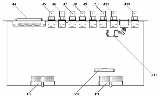
Figure 10-12 A3 Digital IF Assembly Connections - Bottom
