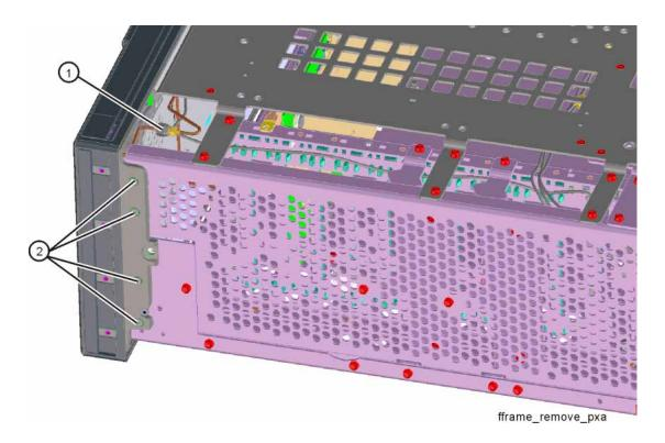
Figure 18-68 Front Panel Cable
