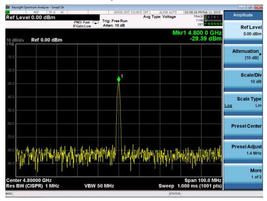
7. If the signal level is not correct refer to Chapter 5, "RF Preselector Section." Chapter 6, "RF Downconverter Section." and Chapter 15, "Block Diagrams." for further troubleshooting information.
