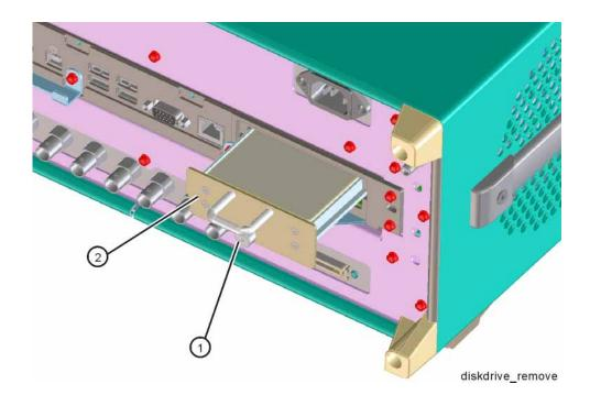
4. Refer to Figure 18-51. Remove the 4 machine screws (1) (0515-0372) from the disk drive carrier assembly that secure the drive (2).
