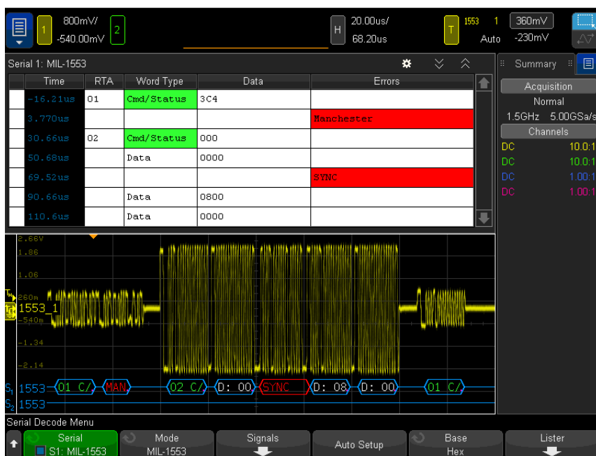
Figure 2. MIL-STD 1553 decode on an InfiniiVision X-Series oscilloscope.
