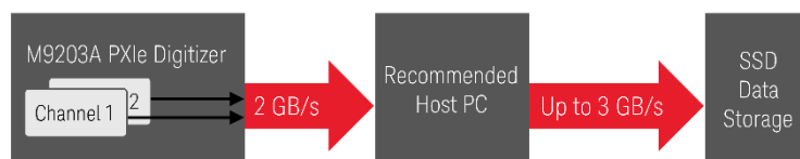
Figure 6. Streaming options (-CB0, -CB2) are proposed with a recommended host PC and SSD. Performance is guaranteed with specific configurations.
