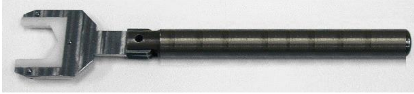
Figure 8. Straightened torque wrench
