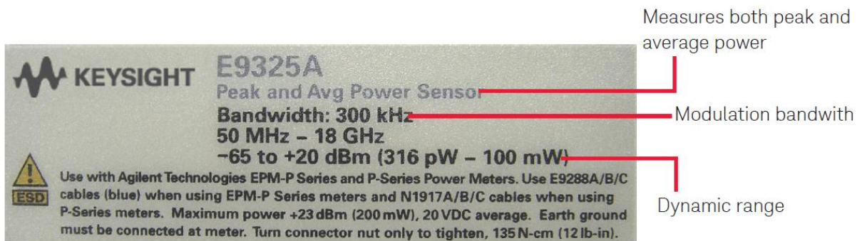
Figure 4. Front label of a diode peak-and-average power sensor
