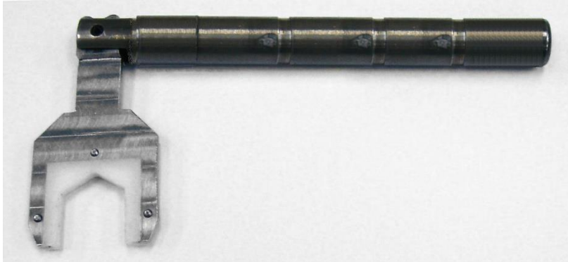
Figure 9. Bent torque wrench
