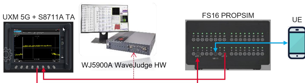
Figure 23. Troubleshooting NTN signaling with WaveJudge
