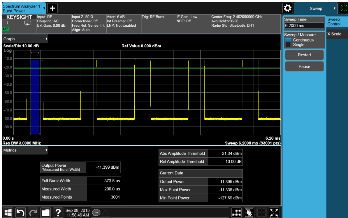
Figure 9-15 Displaying Multiple Bursts
