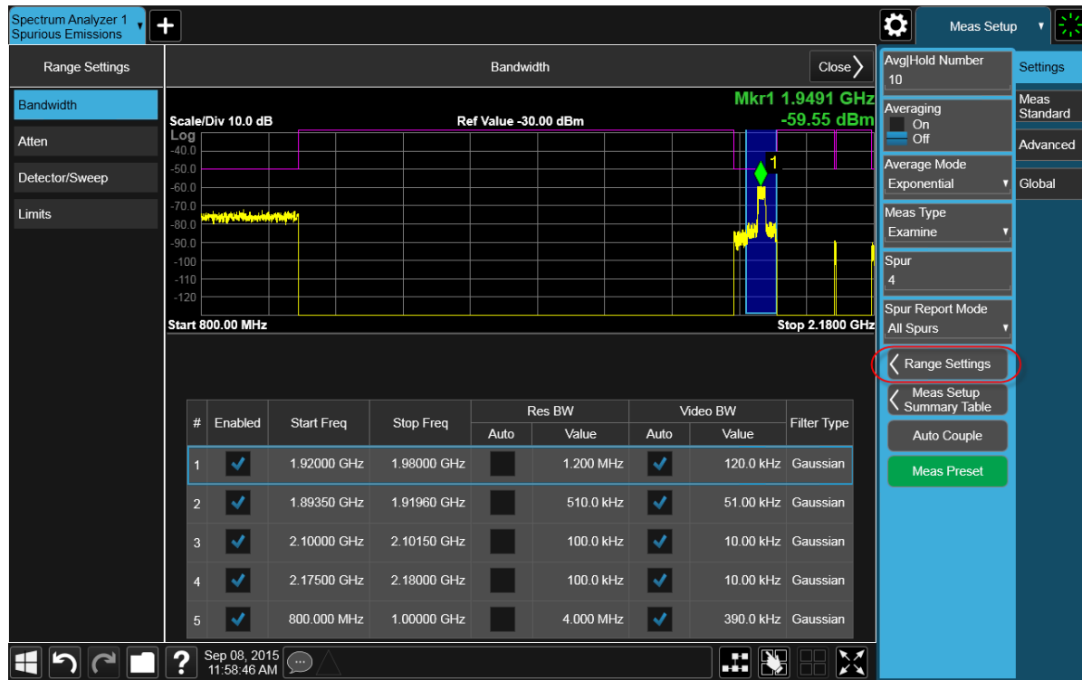
Figure 9-18 Spurious Emission Measurement - Range Settings
