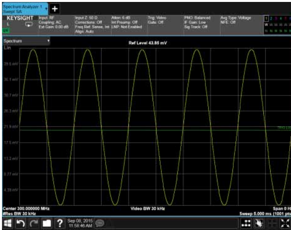
Figure 10-8 AM Signal Measured in the Time Domain
