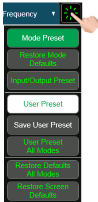
Figure 1-2 Accessing the Preset Panel
