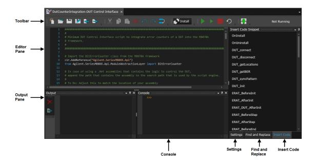
The **DUT Control Interface** interface consists of the following GUI elements:
