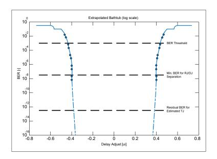
Explanation of the Fast Total Jitter Measurement
