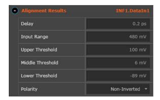
The following figure shows auto-alignment delay results in watt for optical signal in PAM4 mode when the probe is connected:
