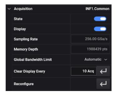
c The channel bandwidth settings are controlled from the Data In **Acquisition** parameters
