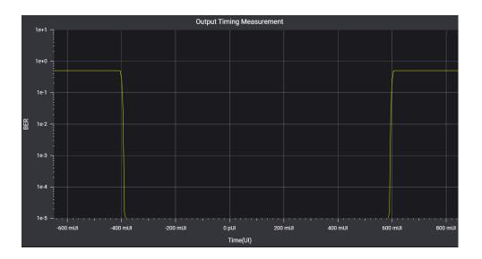
The bathtub curve in the graph shows the overall jitter distribution over a unit interval and serves as the basis for bit error rate estimation.
