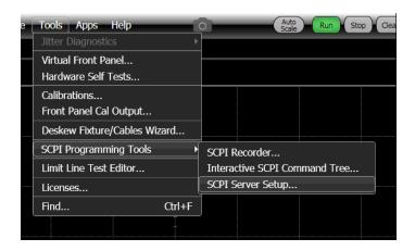
3 Execute the command :EMODulesDCAM1:DEVice "N1076A-US12345678" Select slot number and serial number as required. The example above is using slot 1 (DCAM1) and the serial number US12345678.
