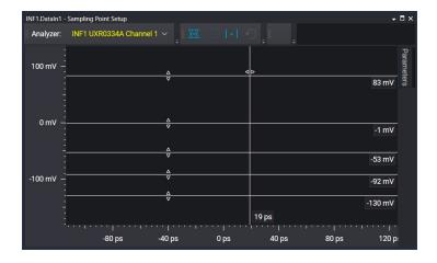
The following image shows the **Sampling Point Setup** window showing PAM8 levels:
