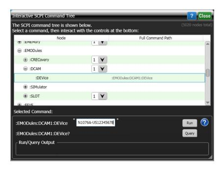
4 Execute the command :EMODules:SLOT1:SELection DCAM Make sure to use the same slot number (1 in this example) as for the previous command.
