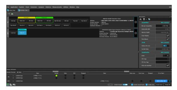
The left side of the figure shows the connected modules and the right side shows the **Parameters** window. The corresponding real-time oscilloscope parameters can be configured through the **Parameters** window.
