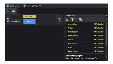
The left side of the figure shows the connected modules, and the right side shows the **Parameters** window. The corresponding real-time oscilloscope parameters can be configured through the Parameters window.
