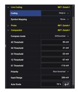
7 The threshold properties are also visible under the 'Alignment Results' functional block.
