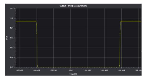
The resulting graph shows you the points in time that have been investigated and whether the actual BER at these points was higher or lower than the BER threshold specified for the measurement.
