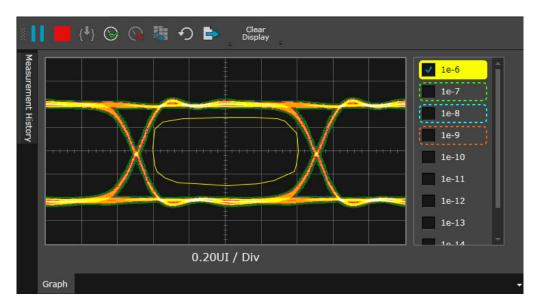
The outer contour represents the measured BER contour, while the inner lines are extrapolated.
