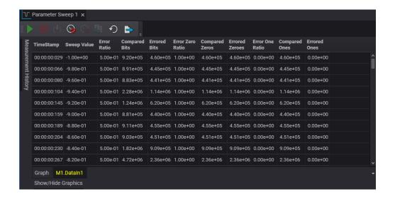
The measurement data displays measurement points such as Sweep Value, Error Ratio, Compared Bits, Errored Bits, Errored Zero Ratio, Compared Zeros, Errored Zeros, Error One Ratio, Compared Ones and Errored Ones which are repeated in the same order for subsequent measured points.
