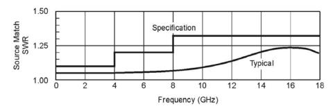
Figure 1 Leveling or ratio measurement source match graph
