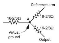
Figure 4 Three-resistor power splitter
