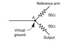
Figure 5 11667A power splitter schematic
