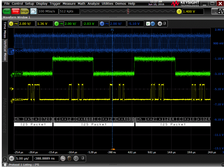
Figure 1. Decoding a TDM I 2 S signal. In this example, 16-bit data (yellow trace) was sent through four channels.
