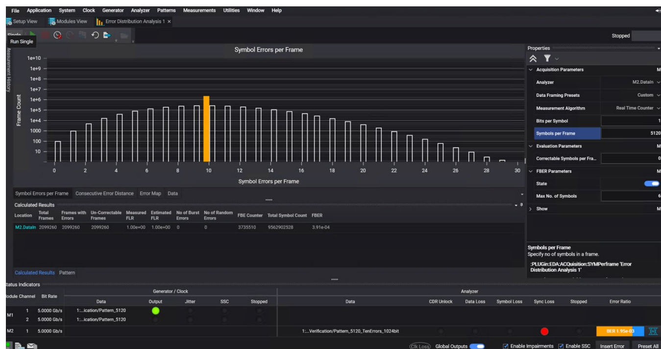
Figure 25. The error distribution analysis M8070EDAB provides multiple views to debug the error distribution. The figure shows an example of symbol errors per frame based on captured pattern streams, with the measured frame loss ratio, based on user-definable number of bits per symbol, correctable symbols per frame and frame length.
