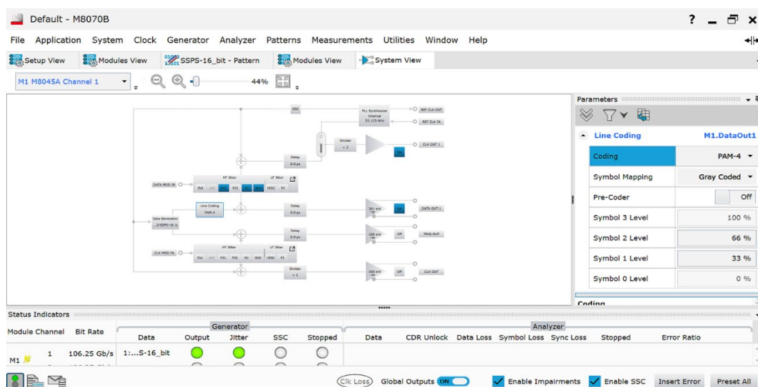
Figure 24. The graphical user interface offers multiple views that can be defined by the user. This example shows the system view on the left side and the pattern generator data output with the PAM4 coding and level linearity parameters at the right.
