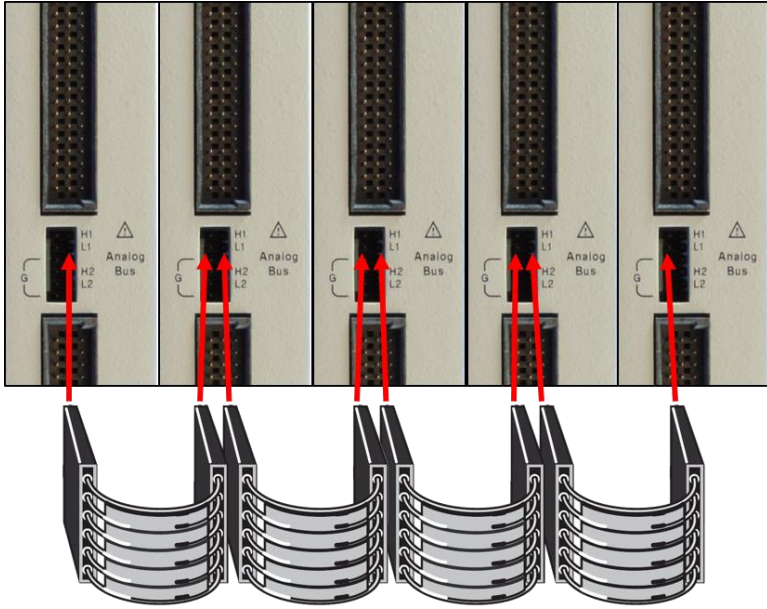
Figure 1. Interconnecting multiple E1460A multiplexers using the analog bus cable
