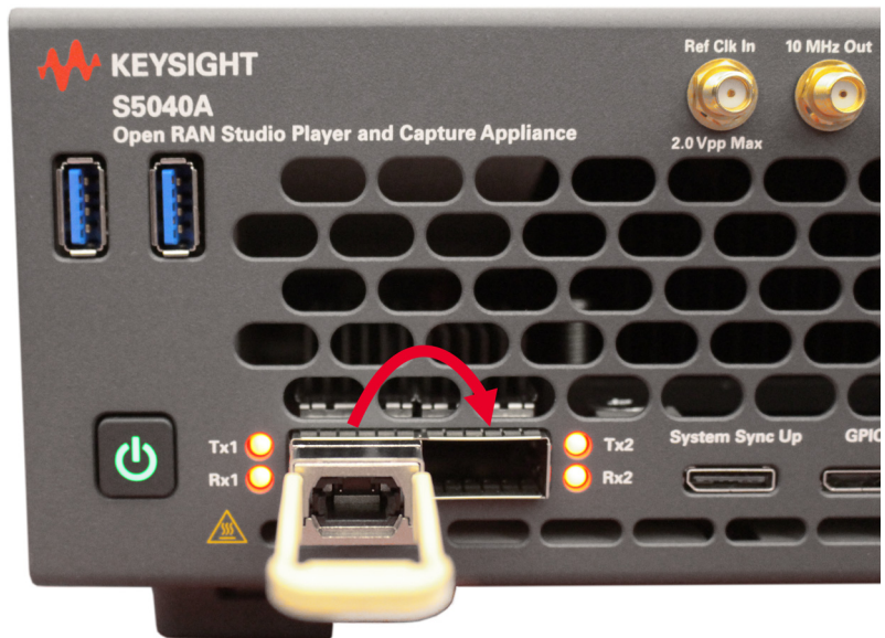
Figure 32 Switching port for QSFP adapter when S5040A Appliance is on
