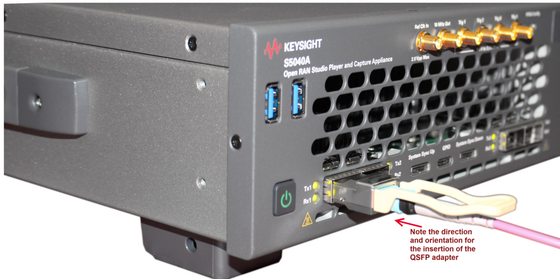
Figure 23 Inserting QSFP28 module into the QSFP port of the S5040A Appliance
