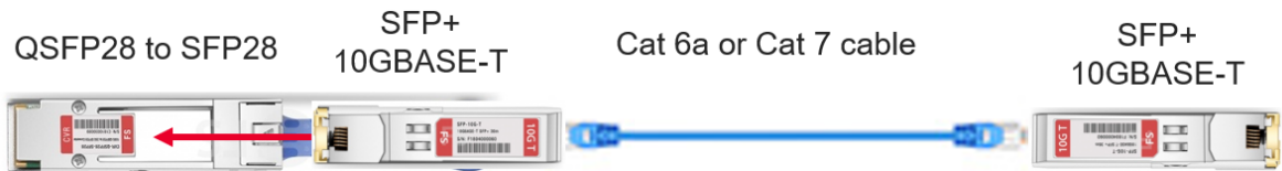
Figure 10 QSFP28 to SFP28 adapter with 10GBASE-T Copper
