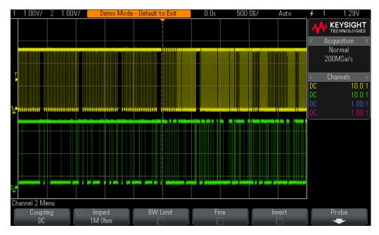
Figure 50 Capturing I<sup>2</sup>C clock and data while triggering on an edge of the clock (channel-1).
