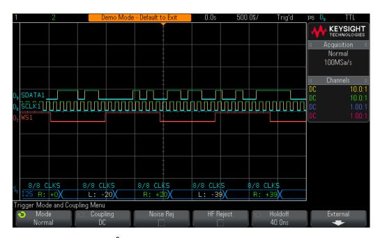
Figure 81 Triggering on  $I^2S$  right-channel = +20.
