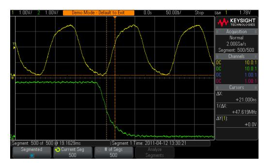
**Figure 43** Using the scope's Segmented Memory acquisition to selectively capture 500 consecutive occurrences of a setup time violationrunt pulses.
