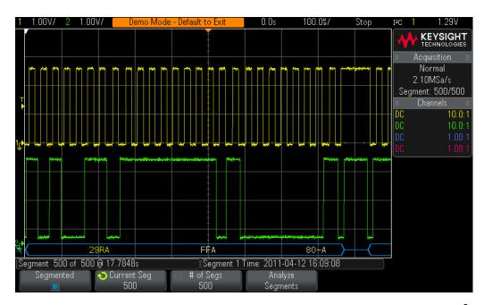
Figure 54 Using the scope's Segmented Memory acquisition to selectively capture more I<sup>2</sup>C traffic.
