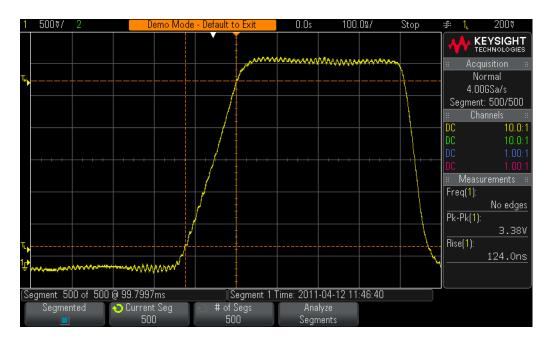
**Figure 35** Using the scope's Segmented Memory acquisition to selectively capture 500 edge violations.
