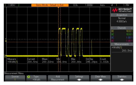
**Figure 9** Measuring the positive pulse width of the 1st pulse in the burst.
