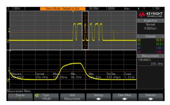
Figure 10 Using the scope's Zoom timebase mode to perform "gated" measurements.
