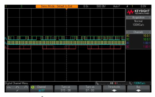
Figure 79 Capturing I<sup>2</sup>S signals using the scope's digital channels of acquisition (MSO).
