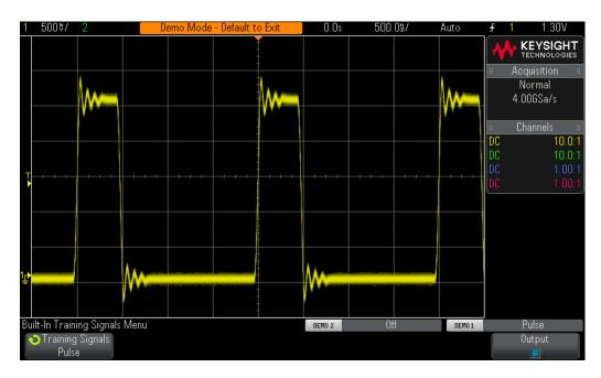
**Figure 1** Oscilloscope setup to capture and display a repetitive digital pulse with ringing and overshoot.
