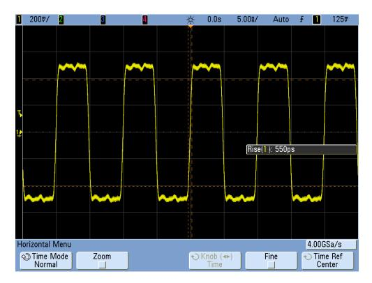
Figure 89 100 MHz digital clock signal captured on a 1 GHz band width scope
