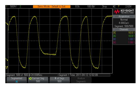
**Figure 40** Using the scope's Segmented Memory acquisition to selectively capture 500 consecutive runt pulses.
