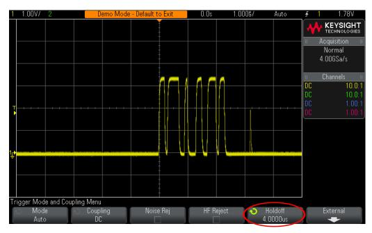
**Figure 8** Setting up the oscilloscope to capture a burst of digital pulses with different pulse widths.
