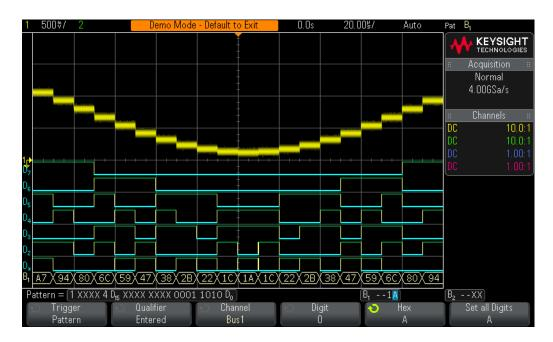
**Figure 49** Triggering on pattern =  $1A_{HEX}$ .
