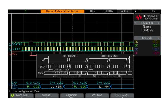
Figure 80 Decoding I<sup>2</sup>S signals.
