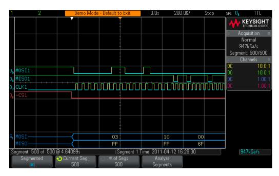
**Figure 59** Using the scope's Segmented Memory acquisition to selectively capture more SPI traffic.
