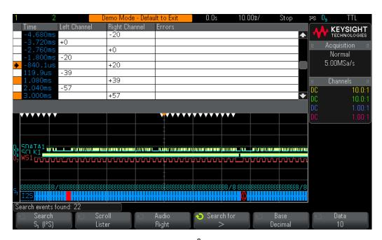
Figure 82 Automatic Search & Navigation on I<sup>2</sup>S data.
