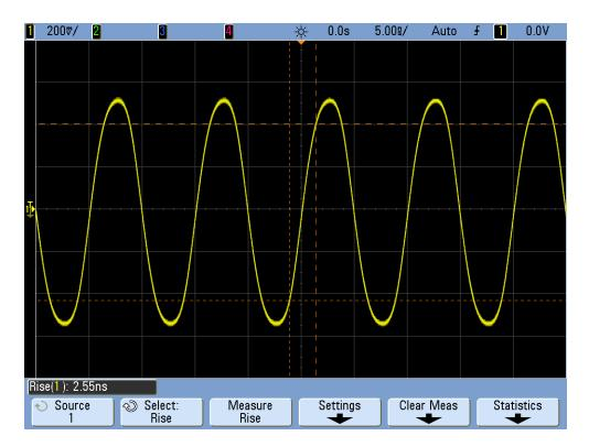
Figure 87 100 MHz digital clock signal captured on a 100 MHz bandwidth scope
