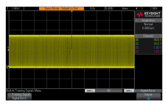
**Figure 22** Attempting to view a burst of pulses while using the scope's default trigger setup conditions.
