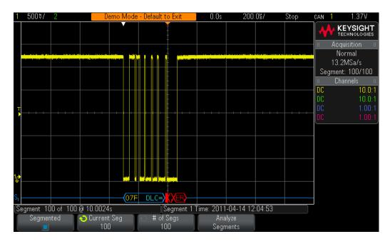
Figure 71 Using the scope's Segmented Memory acquisition to selectively capture 100 CAN error conditions.
