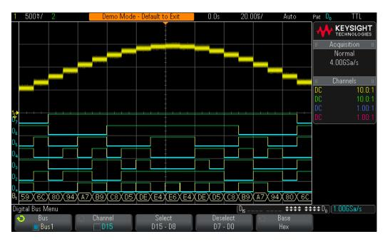
Figure 48 Displaying digital channels in a "bus" display mode.
