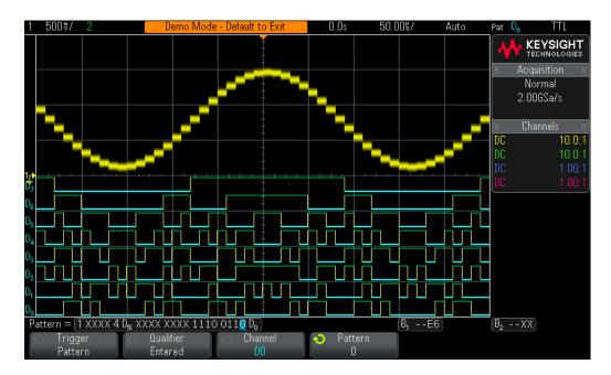
Figure 47 Triggering on Pattern = 1110 0110.
