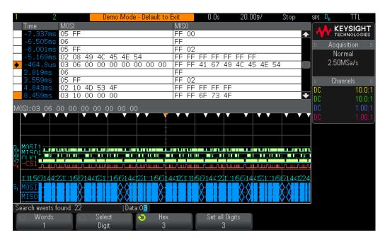
Figure 58 Automatic Search & Navigation on SPI traffic.
