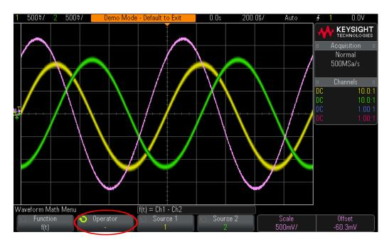
Figure 11 Using waveform math to subtract channel-2 from channel-1.
