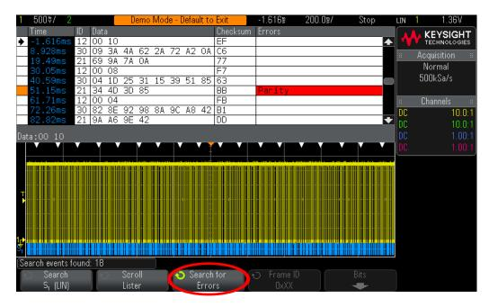
**Figure 76** Using the scope's automatic Search & Navigation capability to find all occurrences of LIN errors over a 2 second time span.
