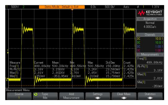
Figure 4 The scope automatically performs up to four parametric measurements.
