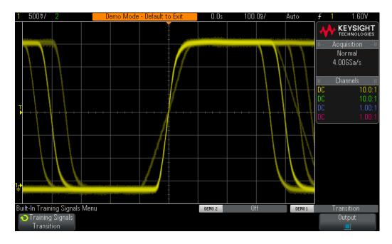
**Figure 31** Scope display reveals two different rising edge speeds when triggering on any rising edge.
