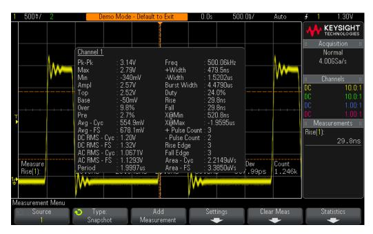
**Figure 7** Performing a comprehensive set of automatic parametric measurements using the "Snapshot All" function.
