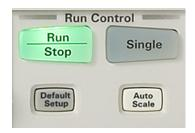
• The [**Default Setup**] key on the front panel sets the oscilloscope to the default configuration.
