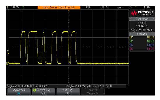
**Figure 28** Using the scope's Segmented Memory acquisition to selectively capture 500 consecutive occurrences of a burst of pulses.
