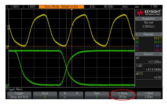
Figure 42 Triggering the scope on just setup time violations of less than 25 ns.
