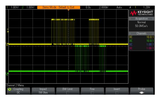
**Figure 60** Capturing RS232/UART transmit and receive data signals using the scope's Edge triggering mode.
