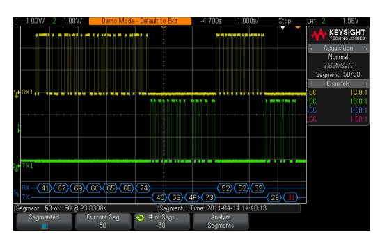
**Figure 65** Using the scope's Segmented Memory acquisition to selectively capture 50 occurrences of Parity Errors.
