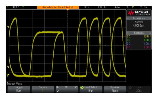
Figure 37 Triggering on positive runts.
