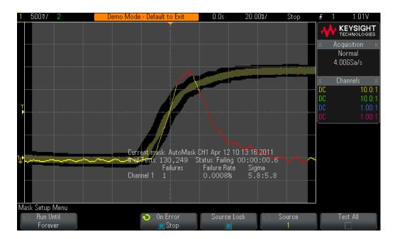
Figure 21 Establishing specific test criteria.
