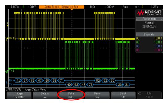
**Figure 62** Triggering on  $Tx = 4D_{HEX}$ .
