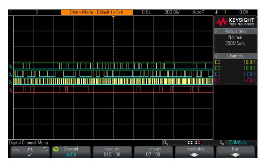
**Figure 55** Capturing 4-wire SPI signals using the scope's digital channels of acquisition (MSO).
