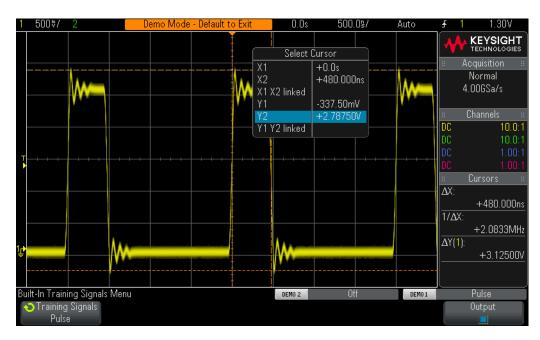
Figure 3 Using the scope's cursor measurements.
