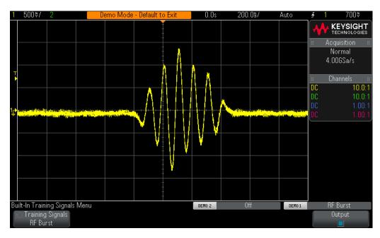
Figure 15 Capturing and displaying an RF burst at 200.0 ns/div.
