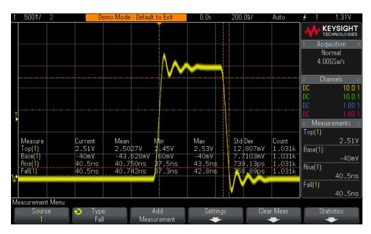
Figure 5 Performing additional pulse parameter measurements on a digital pulse.
