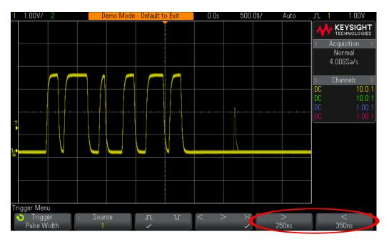
Figure 26 Triggering on a 300 ns wide pulse using the scope's Pulse Width triggering mode.
