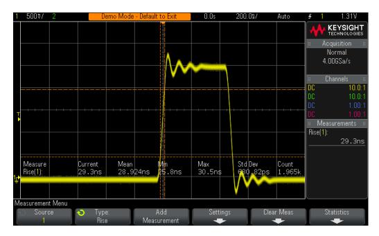
Figure 6 Performing a rise time measurement relative to 20% and 80% threshold levels.
