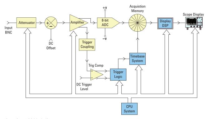
Figure 84 DSO block diagram
