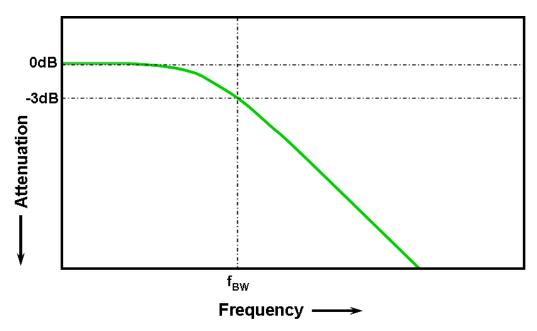
Figure 85 Oscilloscope Gaussian frequency response
