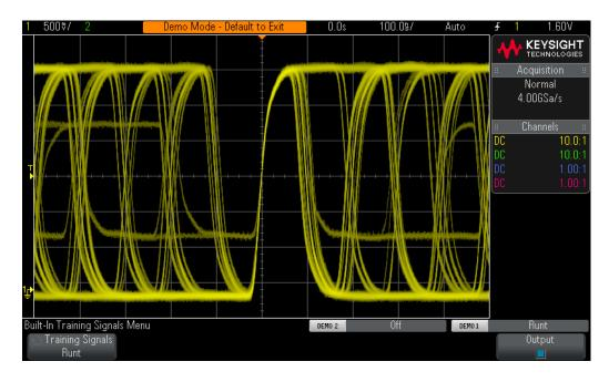
**Figure 36** Scope display reveals various amplitude pulses while triggering on any rising edge.
