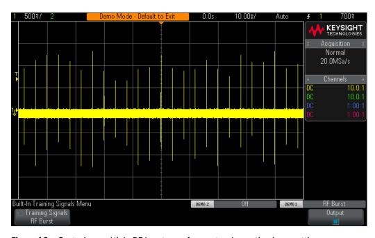
Figure 16 Capturing multiple RF burst waveforms at a slower timebase setting.
