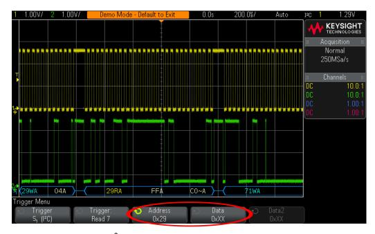
**Figure 52** Triggering on I<sup>2</sup>C traffic.
