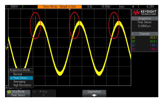
**Figure 14** The Peak Detect acquisition mode reliably captures the narrow glitches riding on the slow sine wave.
