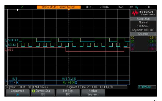
**Figure 83** Using the scope's Segmented Memory acquisition to selectively capture more I<sup>2</sup>S traffic.
