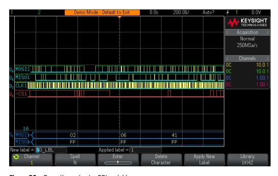
**Figure 56** Decoding a 4-wire SPI serial bus.
