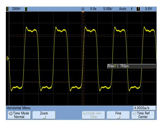
Figure 88 100 MHz digital clock signal captured on a 500 MHz bandwidth scope
