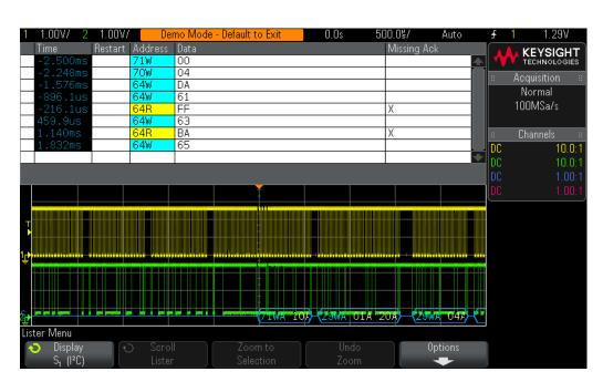
Figure 51 Decoding I<sup>2</sup>C serial bus traffic.
