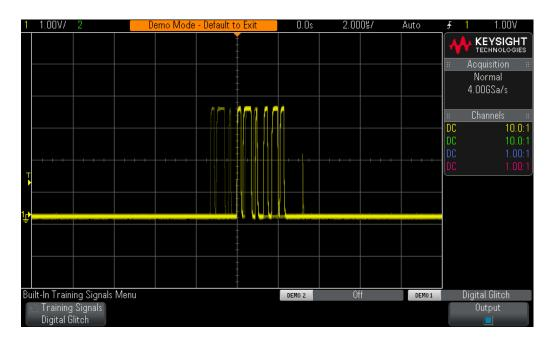
Figure 25 Capturing a digital burst using the scope's default Edge triggering mode.
