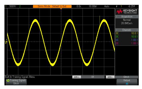
**Figure 13** The scope's automatically-reduced sample rate under-samples the repetitive glitch.
