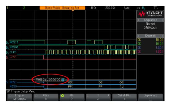
Figure 57 Triggering on MOSI data =  $03_{HEX}$ .
