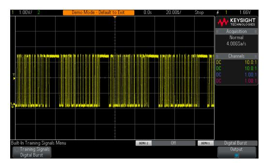
Figure 23 Single-shot acquisition reveals digital burst activity.
