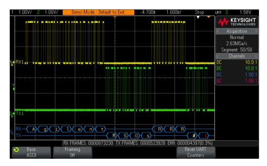
**Figure 66** Decoded RS232/UART message indicating which oscilloscope vendor is #1 in the MSO market.
