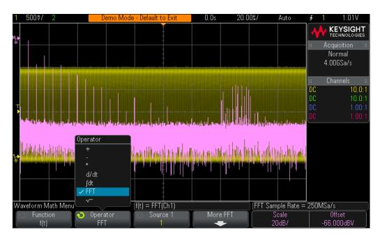
Figure 12 Performing an FFT math function on a repetitive digital clock.
