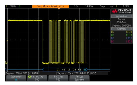
Figure 77 Using the scope's Segmented Memory acquisition to selectively capture 500 LIN frames of a specific ID.
