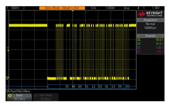
Figure 74 Decoding a LIN bus while triggering on any rising edge of the input signal.
