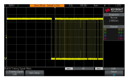
Figure 67 Capturing a CAN frame using the scope's Edge triggering mode.
