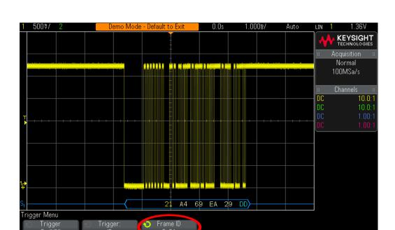
Figure 75 While triggering on LIN frame = 21<sub>HEX</sub>, the scope's hard ware-based decoding reveals parity bit errors in the frame ID field.
