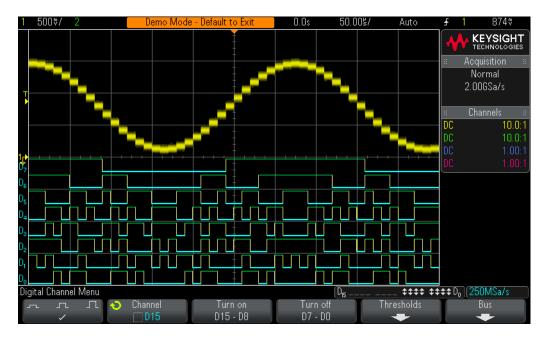
Figure 46 Capturing multiple analog and digital signals with an MSO.
