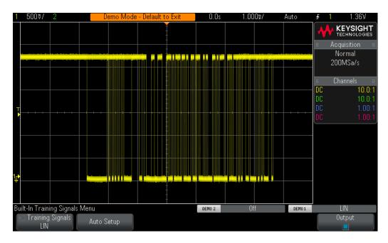
**Figure 73** Capturing a LIN frame using the scope's Edge triggering mode.
