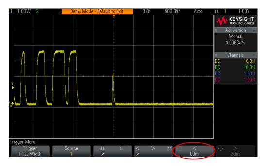
**Figure 27** Triggering on a narrow infrequent glitch using the scope's Pulse Width triggering mode.
