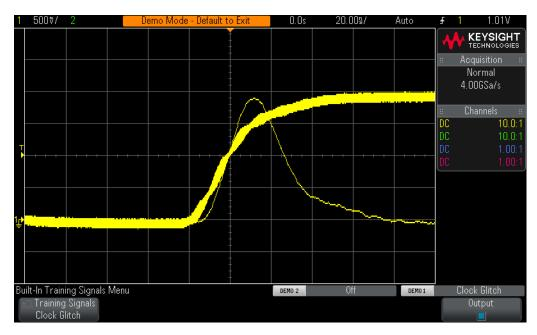
Figure 19 The scope's fast waveform update rate easily captures an infrequent glitch.
