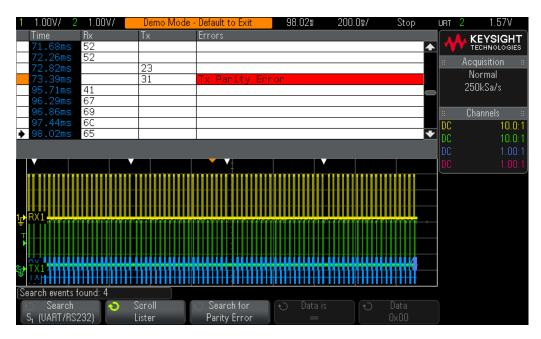
**Figure 63** Using the scope's automatic Search & Navigation capability to find all occurrences of parity bit errors over a 2 second time span.
