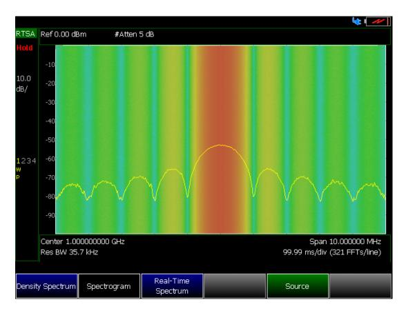
Figure 6. A signal captured using RTSA mode with gap-free results
