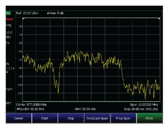
Figure 7. A signal captured using FieldFox's traditional SA mode where the carrier signal masks the interfereing signal
