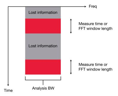
Figure 4. An FFT-based analyzer misses events that occur between time data sample blocks
