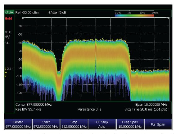
Figure 8. A signal captured using FieldFox's RTSA density display where the interfering signal is seen in the middle of the screen
