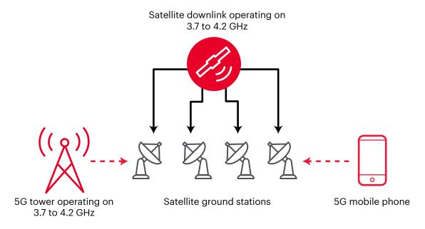
Figure 2. 5G radio tower and mobile phone interfering with satellite ground station communications
