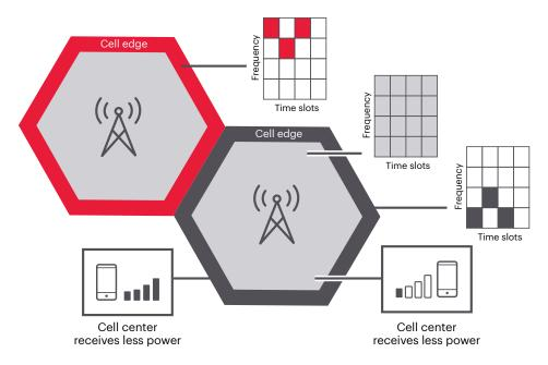
Figure 1. LTE power control and resource block allocation
