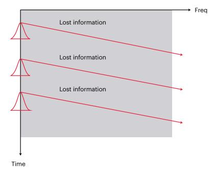
Figure 3. A swept-tuned analyzer misses data events that occur outside the RBW
