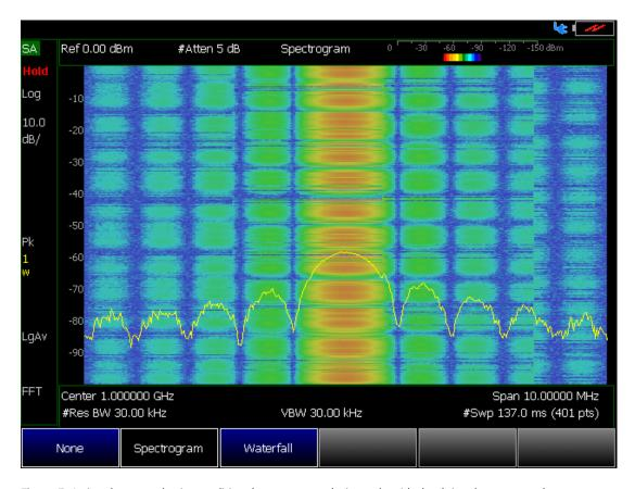
Figure 5. A signal captured using traditional spectrum analysis mode with dead time between updates
