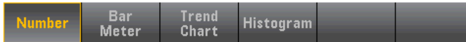
Figure 1. When you press the display button, the soft keys show the choices available for the different display modes
