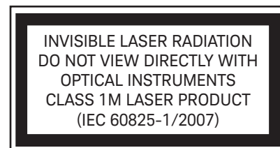
Figure 2. Laser classification label for Class 1M
