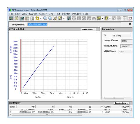
By appending the Id-Vds curve with different VdOff (stress voltage), the current collapse behavior of device can be observed as below.
