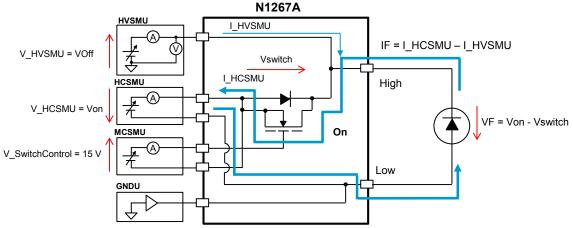
Figure 2-2-7 Relationship of voltage and current at the on-state of diode
