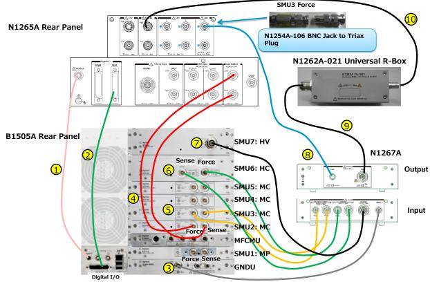
Fig. 4-1-9 Connection between B1505A, N1267A and N1265A (Non-Kelvin)
