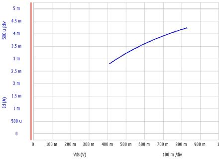
Fig. 4-3-13 Example of Id-Vds curve lower than the maximum current of the HVSMU
