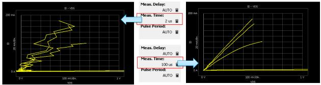
Fig. 4-2-8 Improvement of smoothness by increasing the measurement time
