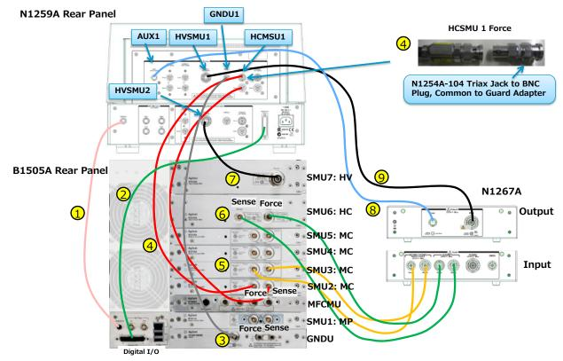
Fig. 4-1-5 Connection between B1505A, N1267A and N1259A (Kelvin)
