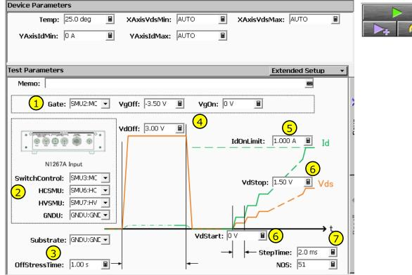
Fig. 4-3-8 Setup parameters for Id-Vds current collapse application test
