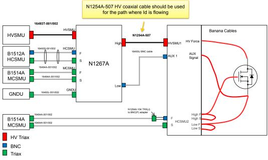
Fig. 4-1-1Wiring diagram of non-Kelvin connection with N1259A
