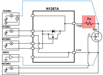
Fig. 3-3-3. Adding series resistance to improve the response time of the HCMSU
