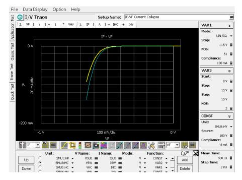
At first, the IF-VF curve without an off-state stress voltage is measured as a reference. This reference has to be measured by clicking the "Measure" button only once (single measurement). In this case, the Source voltage of the HVSMU is set at least 1 V larger than the Stop voltage of the drain voltage sweep (VAR1) to make the diode switch in the N1267A reverse-biased during the off-state of the DUT.
