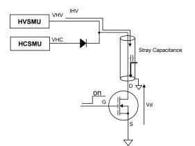
Figure 2-1-3 Unexpected current from the tray capacitance of cabling
