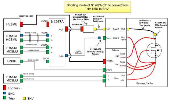
Fig. 4-1-12 Wiring diagram of Kelvin connection with N1259A
