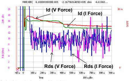
Fig. 3-4-8 Example of transient of the HVSMU
