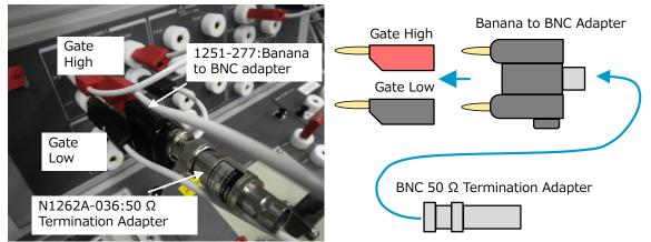
(b) Inserting 50  $\Omega$  resistor to the Gate drive
