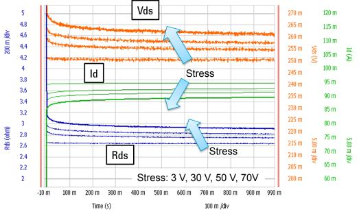
Fig. 4-4-17 Overlaid results with varying stress voltage
