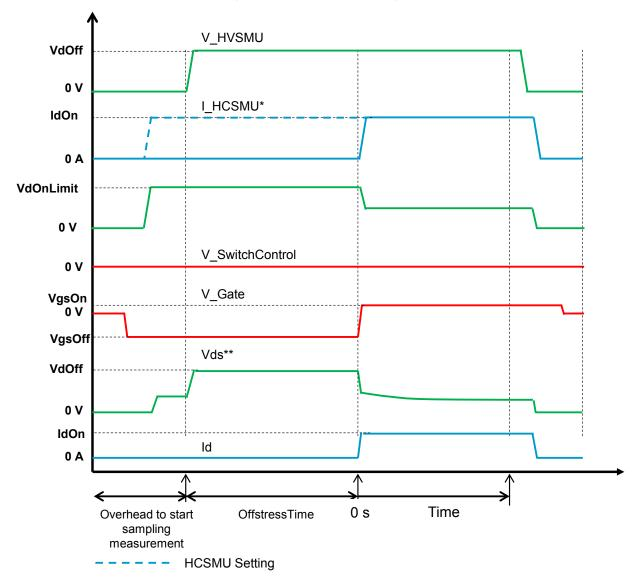
Order to output voltage: Substrate  $\rightarrow$  Switch Control  $\rightarrow$  Gate  $\rightarrow$  HCSMU  $\rightarrow$  HVSMU
