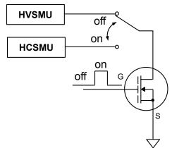
Fig. 1-3 Switching of the HVSMU and HCSMU synchronized with device
