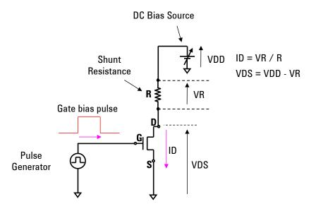
Fig. 3-1-4 Dynamic Ron measurement system using a shunt resistor
