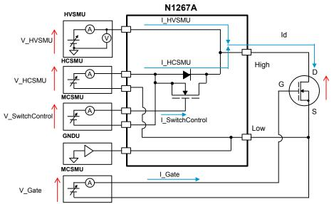
Figure 2-1-6 Block diagram of the N1267A
