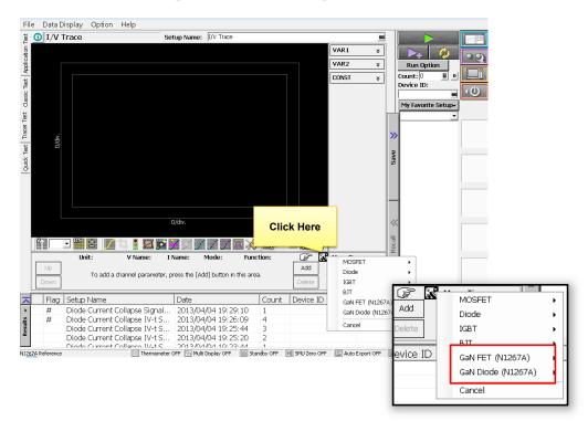
In those preset groups, there are two categories of measurements, IV characteristic measurement to check the DUT adequateness and current collapse measurement.
