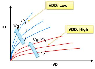
Fig. 1-2 Current Collapse of GaN FET
