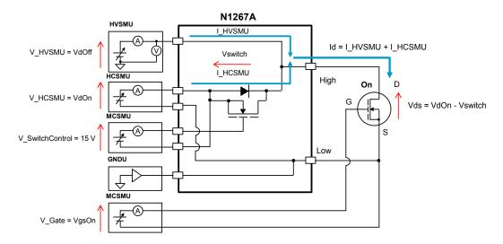
Fig. 3-4-5 Current and voltage when device is turned on
