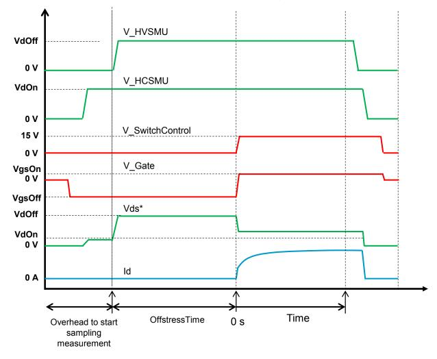
Order to output voltage: Substrate  $\rightarrow$  Switch Control  $\rightarrow$  Gate  $\rightarrow$  HCSMU  $\rightarrow$  HVSMU \*: Vds at on-state is higher than the "VdOn" due to the voltage drop at the switch inside of the N1267A.
