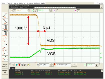
Fig. 3-2-1 Waveform from the off-state to the on-state
