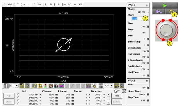
Fig. 4-4-3 Performing interactive spot measurement
