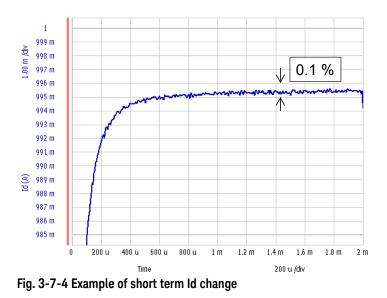
From these examples, it is possible to say the Id can be used to monitor the current collapse in short term measurement. But for long term measurement, the Rds should be used if the Id is larger than 100 mA.
