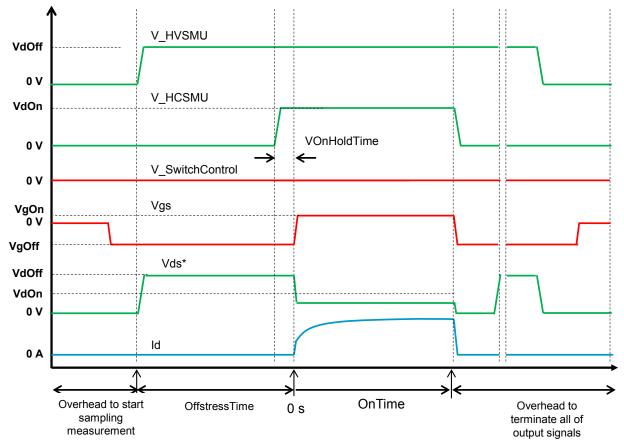
Order to output voltage: Substrate  $\rightarrow$  Switch Control  $\rightarrow$  Gate  $\rightarrow$  HCSMU  $\rightarrow$  HVSMU \*: Vds at on-state is lower than the "VdOn" due to the voltage drop at the switch inside of the N1267A.
