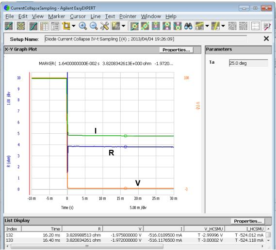
\*This sample device is a Si diode and does not have any current collapse characteristics.
