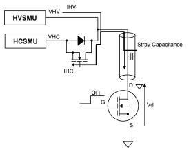
Fig. 2-1-4 Discharge the stray capacitance through the switch
