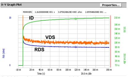
Figure 3-1-2 is an example of dynamic Ron measurement in GaN FET
