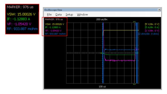
The IF is a combination of the current measured by the HCSMU and HVSMU. The VF is a measured voltage by the HVSMU. The RF is calculated from the measured VDS and ID.
