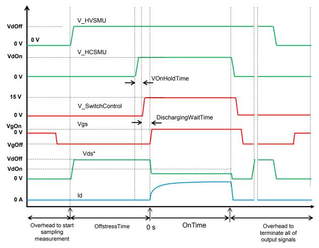
Order to output voltage: Substrate  $\rightarrow$  Switch Control  $\rightarrow$  Gate  $\rightarrow$  HCSMU  $\rightarrow$  HVSMU \*: Vds at on-state is higher than the "VdOn" due to the voltage drop at the switch inside of the N1267A. [Measurement Timing]
