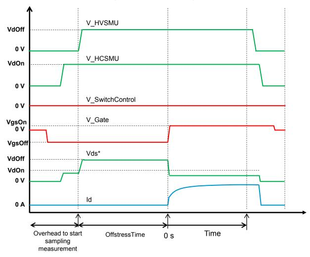
Order to output voltage: Substrate  $\rightarrow$  Switch Control  $\rightarrow$  Gate  $\rightarrow$  HCSMU  $\rightarrow$  HVSMU \*: Vds at on-state is lower than the "VdOn" due to the voltage drop at the switch inside of the N1267A.
