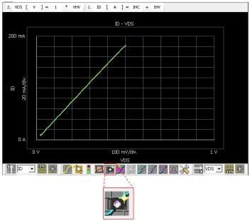
Fig. 4-3-4 Capture ID-VDS curve as a reference
