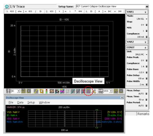
Fig. 4-4-22 Enabling the Oscilloscope View
