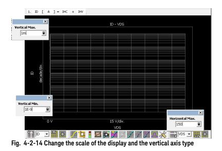
In this case, since the VDSS of the DUT is 120 V, 150 V is selected as the maximum value of the horizontal scale including some margin of the spec.
