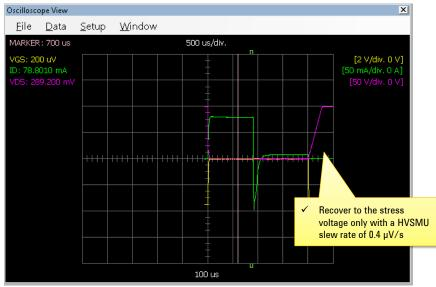
Fig. 3-4-9 Slow recovery of the HVSMU from the on-state to the off-state
