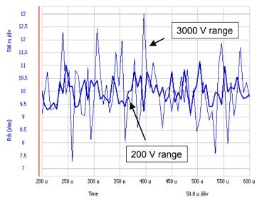
Fig. 3-8-1 Repeatability of measured Rds by stress voltage
