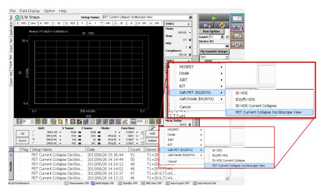
Fig. 3-5-6 FET current collapse measurement pre-set in the Tracer Test Mode
