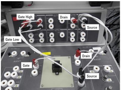
(a) Twisting measurement cables
