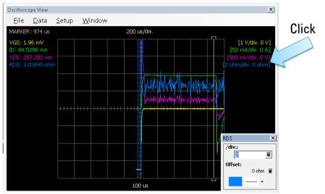
Fig. 4-4-24 Changing the vertical scale of each waveform
