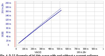
Fig. 4-3-11 Example of Id-Vds curve with and without a current collapse
