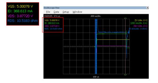
The ID is a combination of current measured by the HCSMU and HVSMU. The VDS is a measured voltage by the HVSMU. RDS is calculated from the measured VDS and ID.
