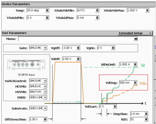
Fig. 4-3-14 Measurement setup to get result of figure 4-3-13
