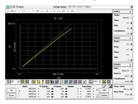
This setup measures the Id-Vds curve at the gate bias voltage specified as the Stop voltage of the VAR2 parameter. The Start voltage of the VAR2 sweep is the gate voltage to make FET turned off. Off-state stress voltage is specified as the Source voltage of the HVSMU.
