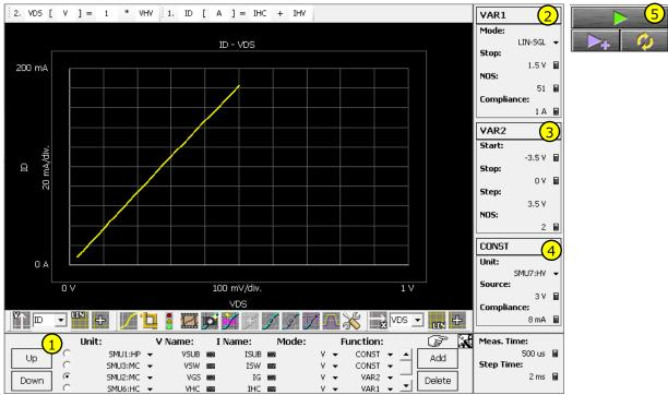
Fig. 6-3-2 Step to measure the reference ID-VDS curve
