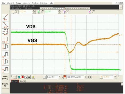
(b) Waveform captured by the Oscilloscope (VSW: 20 µs width, 86 µs delay)
