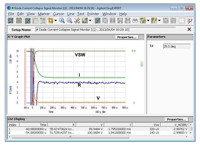
\*: The voltage at the on-state is higher than "Von" due to the voltage drop at the switch inside of the N1267A when I is larger than the current compliance of the HVSMU. If I is smaller than the current compliance of the HVSMU, V becomes larger than Von.
