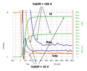
Fig. 3-4-2 Delay of voltage measurement by HVSMU
