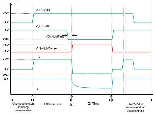
Order to output voltage: Substrate→Switch Control→ HCSMU→HVSMU \*: The voltage at the on-state is higher than "Von" due to the voltage drop at the switch inside of the N1267A
