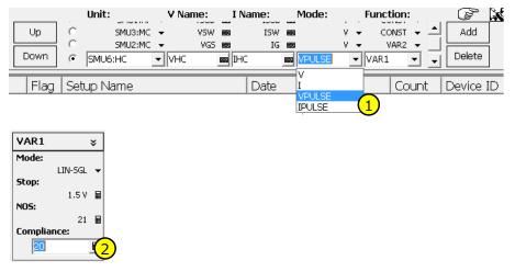
Fig. 4-3-7 Changing operation mode to the "VPULSE" mode.
