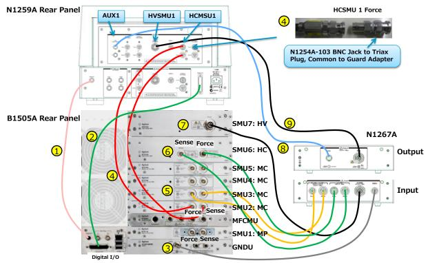
Fig. 4-1-2 Connection between B1505A, N1267A and N1259A (Non-Kelvin)
