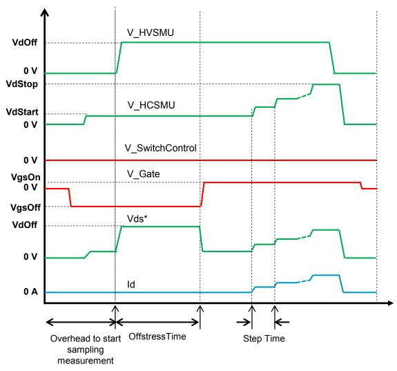
Order to output voltage: Substrate $\rightarrow$ Switch Control $\rightarrow$  Gate $\rightarrow$  HCSMU $\rightarrow$ HVSMU \*: The Vds at on-state is higher than the "VdOn" due to the voltage drop at the switch inside of the N1267A Case 2: DischargeSwitchControl is "On"
