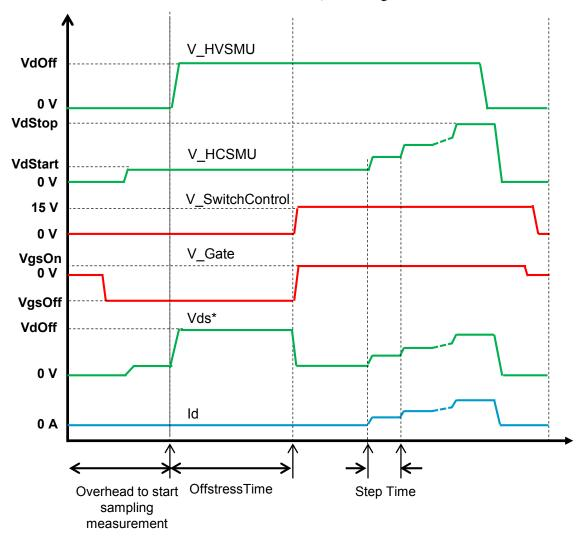
Order to output voltage: Substrate $\rightarrow$ Switch Control $\rightarrow$  Gate $\rightarrow$  HCSMU $\rightarrow$ HVSMU \*: The Vds at on-state is smaller than the "VdOn" due to the voltage drop at the switch inside of the N1267A
