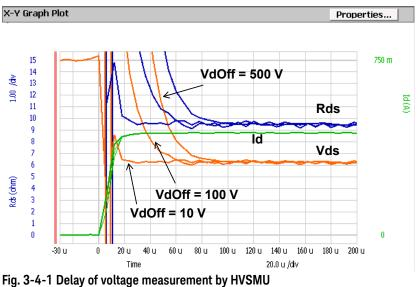
From this example, the settling time of the measured drain voltage (Vds) is getting longer along with the increase of the VdOff.
