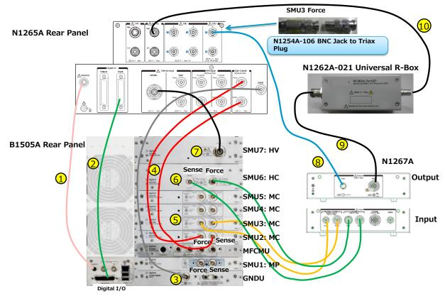
Fig. 4-1-13 Connection between B1505A, N1267A and N1265A (Kelvin)
