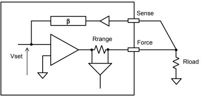
Fig. 3-3-1 Simplified Circuit Diagram of the HCMSU
