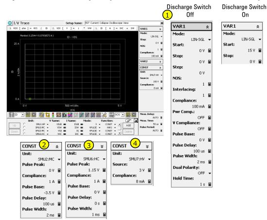
Fig. 4-4-21 Example setup to measure the reference data
