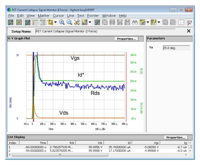
\*The step on the Id is due to the overcurrent status of the HVSMU (12 mA). Please refer to section 3, "Switching Performance".
