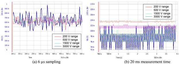
Figure 3-8-2 shows the example of voltage measurement repeatability by HVSMU in different measurement times.
