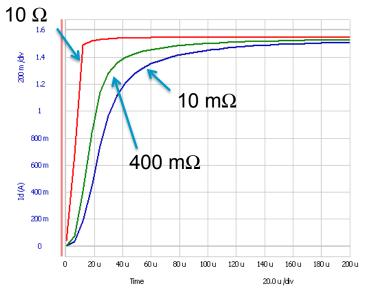
Fig. 3-3-2 Step response of measured current by HCSMU
