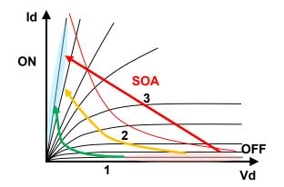
Figure 2-1-5 Transient path from the off-state to the on-state
