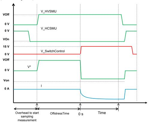
Order to output voltage: Substrate $\rightarrow$ Switch Control $\rightarrow$  HCSMU $\rightarrow$ HVSMU
