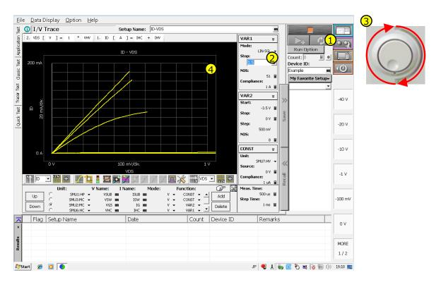
Fig. 4-2-6 Verifying Id-Vds characteristics by interactive operation of the Tracer Test mode
