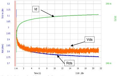
Fig. 3-7-2 Example of Current Collapse Measurement
