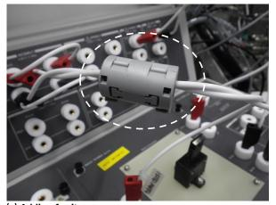
(c) Adding ferrite core Fig. 4-2-10 Examples of techniques to stop device oscillation
