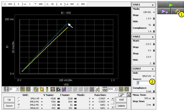
Fig. 4-3-6 Observing a recovery from the current collapse situation
