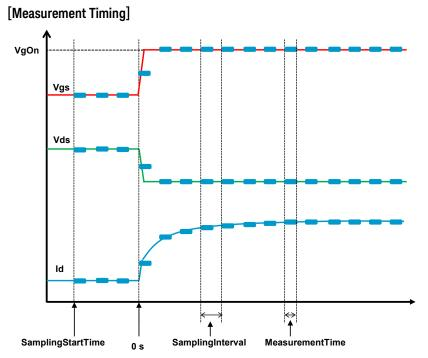
\*If the MeasurementTime is longer than SamplingInterval, measurement points during the MeasurementTime are skipped.
