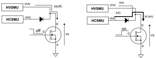
Fig. 2-1-1. How the diode switch works in N1267A
