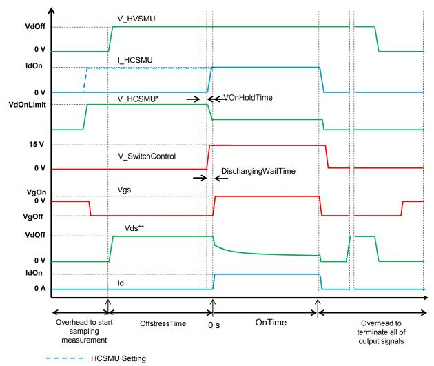
Order to output voltage: Substrate  $\rightarrow$  Switch Control  $\rightarrow$  Gate  $\rightarrow$  HCSMU  $\rightarrow$  HVSMU
