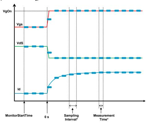
$\ast$  Minimum sampling interval is 6  $\mu s.$  Sampling Interval and Measurement Time are adjusted automatically by the "MeasurementDuration".
