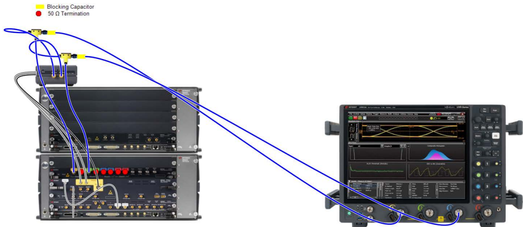
Figure 30 Example connection diagram for ASIC and CEM direct-connection calibrations, 8.0 GT/s and above (TP1, 4-channel UXR, M8050A)
