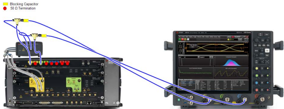
Figure 29 Example connection diagram for ASIC and CEM direct-connection calibrations, 8.0 GT/s and above (TP1, no TTC, 4-channel UXR, M8040A)
