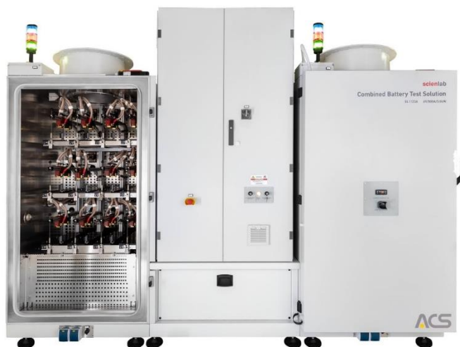
Figure 2. Left: Cell holders for 12 prismatic cells in each chamber.
