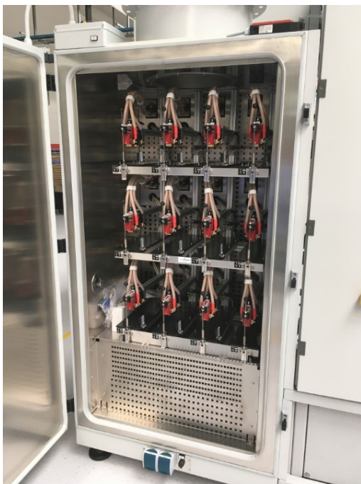
Cell holders for 12 prismatic cells in each chamber.
