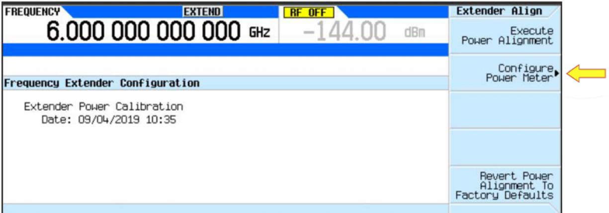
Figure 21 Configure Power Meter
