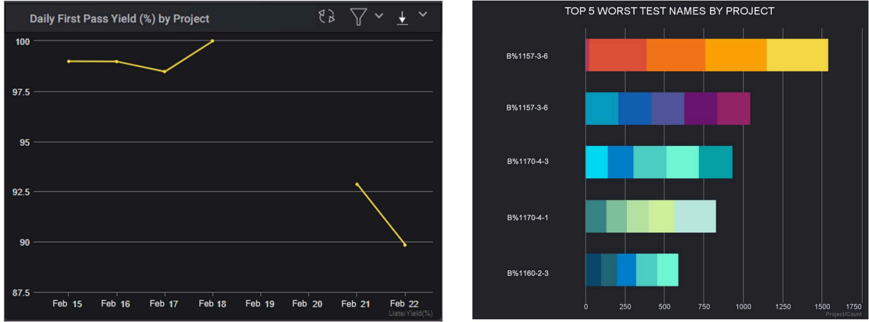
Figure 3. Daily FPY by project and corresponding worst tests for each project to help drive investigations into the failures.
