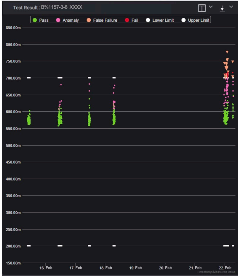
Figure 2. Corresponding measurement chart showing the eventual failures that affected the FPY as the volume of anomalies started to rise on 18-Feb and started to fail on 22-Feb (triangles show the retest passing boards).
