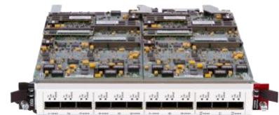
Xcellon-Multis Reduced 1-slot, 12-port load module
