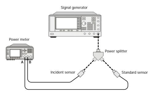
Figure 2-3 Equipment setup for low power verification
