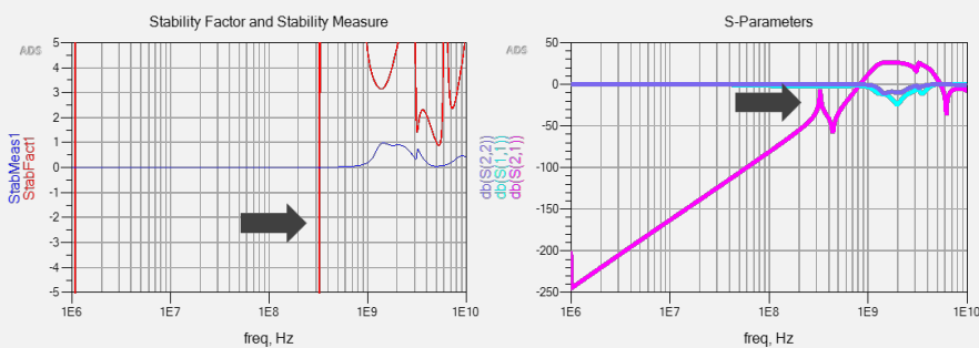
Figure 50. Adding a bondwire to the bias causes K-factor to drop with negative Stability Measure (left), resulting in a corresponding spike seen in the S(2,1) response (right).
