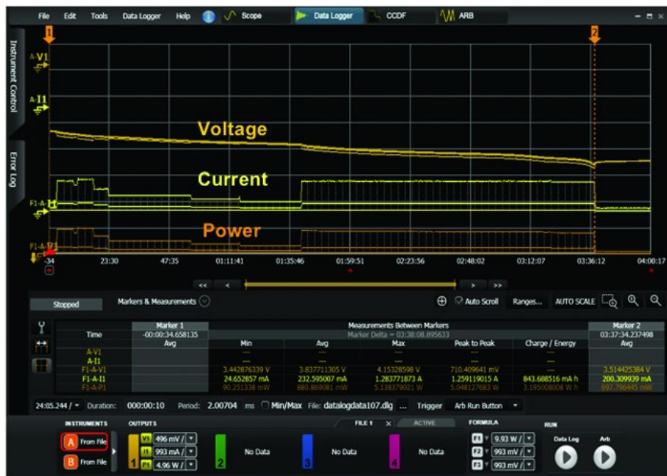
Figure 6. Data logging acquisition showing voltage, current, and power (actual battery rundown)
