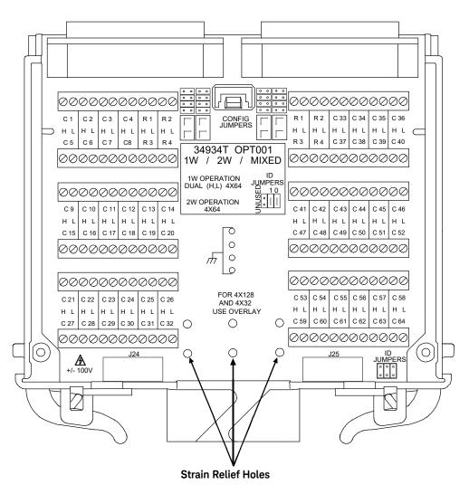
Note the six strain relief holes provided in the terminal block PCB. See the following page for instructions on providing wiring strain relief.
