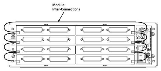
Eight 34934A modules (with attached configuration blocks) connected in an extended-row configuration.
