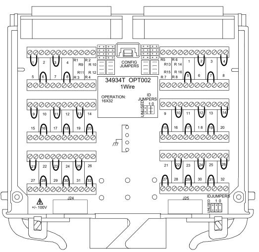
Once these jumpers are placed, you can make column connections to the column terminals which remain open.
