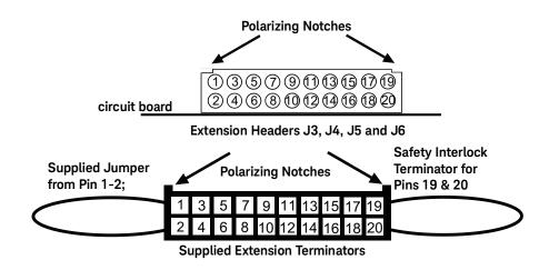
You must fabricate custom cabling to make row signal connections to the central 16 pins (3-18) of these headers, using the pin assignments below. The supplied blue terminators accommodate 22 AWG coated wire, fitted to "crimp-to-wire" contacts with latch tabs.
