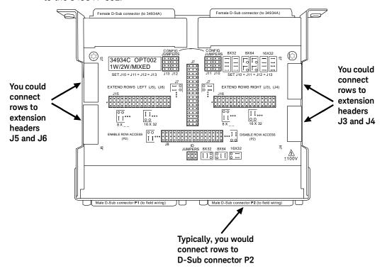
Typically, you could make both row and column connections to each module by fabricating custom cabling terminating in female D-Sub connectors. These attach to the configuration block's male D-Sub connectors P1 and P2. For 16x32, all rows connect to P2.
