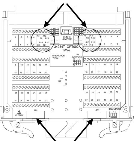
You can connect row signals to the screw terminals here...
