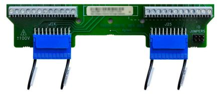
The supplied terminators incorporate both the shorting jumper for pins 19 and 20 and a jumper precluding connection to pins 1 and 2. Detailed pin diagrams for these terminators are provided on page 229.
