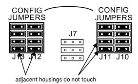
When installing the Config Jumpers ensure that the adjacent housing do NOT touch! Failure to do so may result in hazardous conditions such as fire or shock and could lead to personal injury or death.
