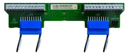
The supplied terminators incorporate both the shorting jumper for pins 19 and 20 and a jumper precluding connection to pins 1 and 2. Detailed pin diagrams for these terminators are provided on page 164.
