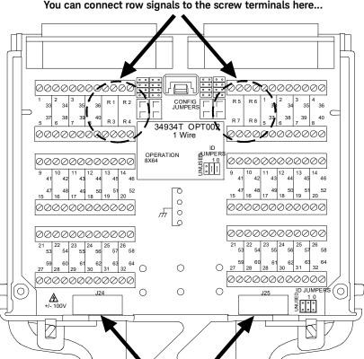
You can connect row signals to the screw terminals here...
