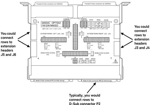
Typically, you could make both row and column connections to each module by fabricating custom cabling terminating in female D-Sub connectors. These attach to the configuration block's male D-Sub connectors P1 and P2. For 8x64, all rows connect to P2.
