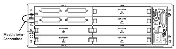
Two 34934A modules (with attached configuration blocks) connected in an extended-row configurati
