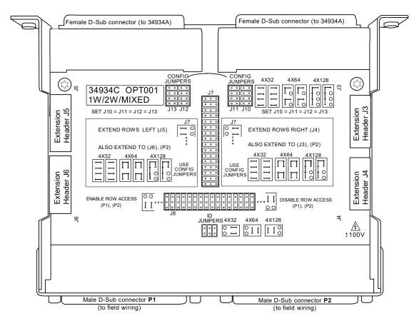
Note four types of on-board jumpers you'll have to set to configure this board; some will be familiar from the configuration descriptions of the *terminal blocks*, but some are new. Instructions for setting these are provided in "34934C-001 Configuration Block: 4x64 Jumper Configuration" on page 106.
