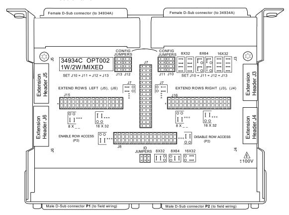
Note five types of on-board jumpers you'll have to set to configure this board; some will be familiar from the configuration descriptions of the *terminal blocks*, but some are new. Instructions for setting these are provided in "34934C-002 Configuration Block: 16x32 Jumper Configuration" on page 233.
