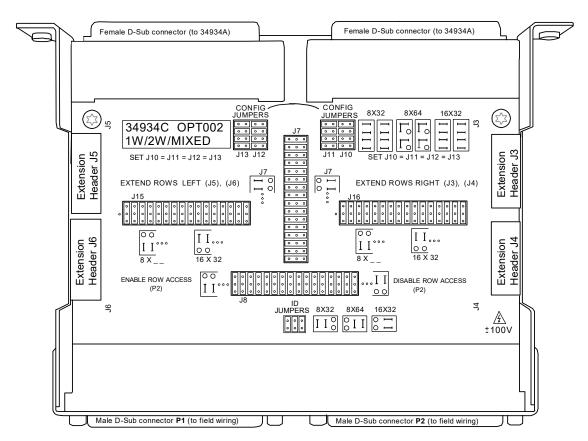
Note five types of on-board jumpers you'll have to set to configure this board; some will be familiar from the configuration descriptions of the *terminal blocks*, but some are new. Instructions for setting these are provided in "34934C-002 Configuration Block: 8x64 Jumper Configuration" on page 199.
