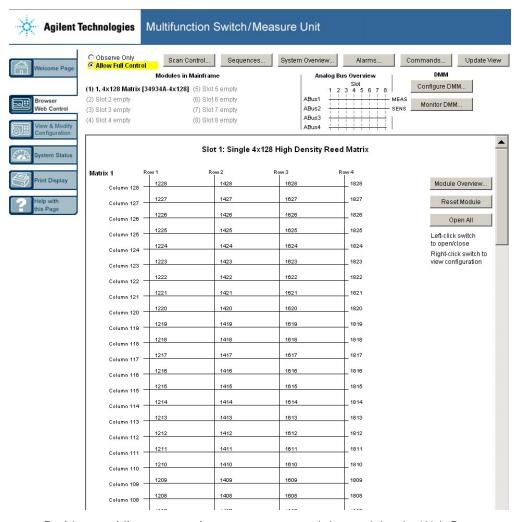
Besides providing a convenient means to control the module, the Web Browser offers the easiest method to view the channel map for any set configuration of the module.
