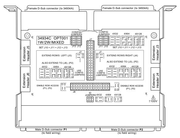
Note four types of on-board jumpers you'll have to set to configure this board; some will be familiar from the configuration descriptions of the *terminal blocks*, but some are new. Instructions for setting these are provided in "34934C-001 Configuration Block: 4x32 Jumper Configuration" on page 72.
