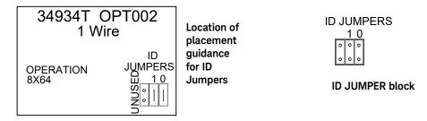
To set the correct ID code for 8x64, place two vertically positioned jumpers as shown below.
