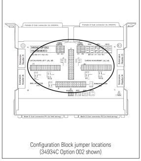
When setting the configuration jumpers for the desired 34934A matrix configuration and the additional row extension and row access jumpers on the Configuration Block, use cotton gloves while handling the individual jumpers. Once the jumpers are set, adjust their position such that adjacent jumpers are not in contact with one another. The figures on the following page show this positioning.
