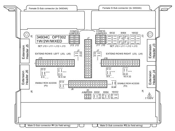
Note five types of on-board jumpers you'll have to set to configure this board; some will be familiar from the configuration descriptions of the *terminal blocks*, but some are new. Instructions for setting these are provided in "34934C-002 Configuration Block: 8x32 Jumper Configuration" on page 168.
