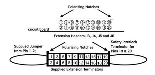
You must fabricate custom cabling to make row signal connections to the central 16 pins (3-18) of these headers, using the pin assignments below. The supplied blue terminators 34934-80006 accommodate 22 AWG coated wire, fitted to "crimp-to-wire" contacts with latch tabs.
