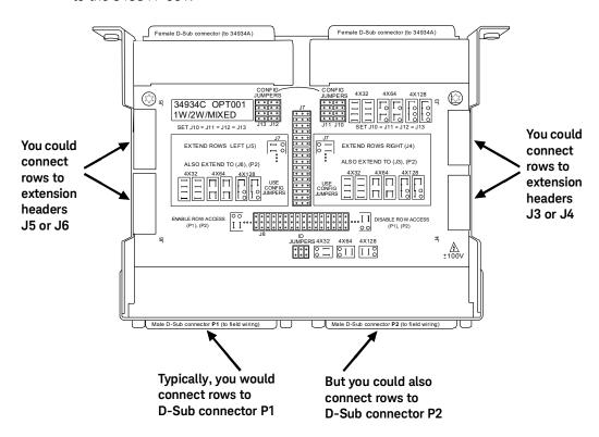
Typically, you could make both row and column connections to each module by fabricating custom cabling terminating in female D-Sub connectors. These attach to the configuration block's male D-Sub connectors P1 and P2.
