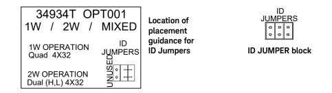
To set the correct ID code for 4x32, place two horizontally positioned jumpers as shown below.
