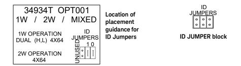
To set the correct ID code for 4x64, place two vertically positioned jumpers as shown below.
