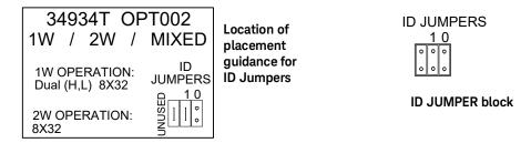
To set the correct ID code for 8x32, place two vertically positioned jumpers as shown below.
