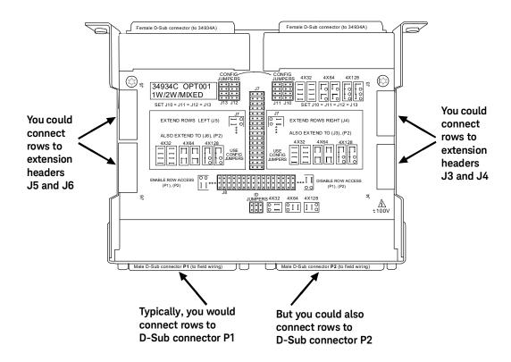
Typically, you could make both row and column connections to each module by fabricating custom cabling terminating in female D-Sub connectors. These attach to the configuration block's male D-Sub connectors P1 and P2.
