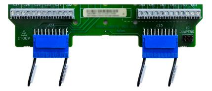
The supplied terminators incorporate both the shorting jumper for pins 19 and 20 and a jumper precluding connection to pins 1 and 2. Detailed pin diagrams for these terminators are provided on page 104.
