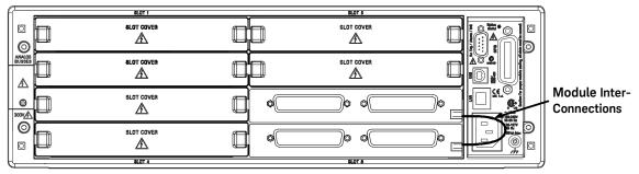
Alternate method of connecting two 34934A modules.
