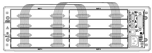
Eight 34934A modules (with attached terminal blocks) connected in an extended-row configuration.
