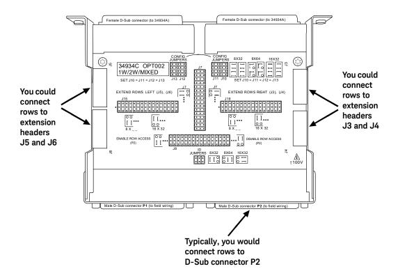
Typically, you could make both row and column connections to each module by fabricating custom cabling terminating in female D-Sub connectors. These attach to the configuration block's male D-Sub connectors P1 and P2. For 8x32, all rows connect to P2.
