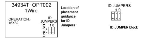
To set the correct ID code for 16x32, place two horizontally positioned jumpers as shown below.
