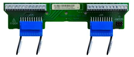
The supplied terminators incorporate both the shorting jumper for pins 19 and 20 and a jumper precluding connection to pins 1 and 2. Detailed pin diagrams for these terminators are provided on page 195.
