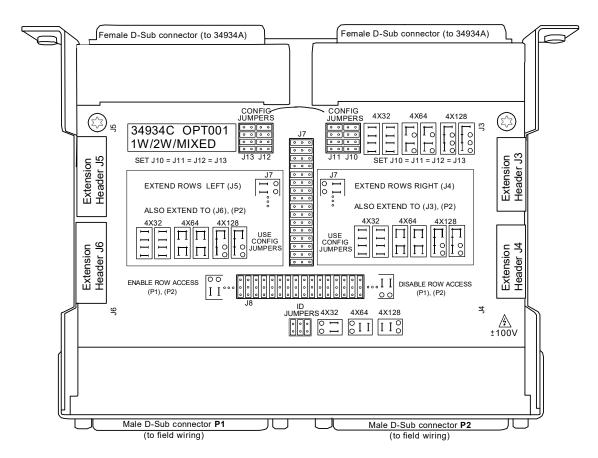
Note four types of on-board jumpers you'll have to set to configure this board; some will be familiar from the configuration descriptions of the *terminal blocks*, but some are new. Instructions for setting these are provided in "34934C-001 Configuration Block: 4x128 Jumper Configuration" on page 137.
