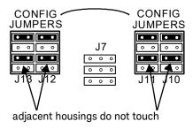
2 Then stack eight vertically positioned jumpers as shown below.
