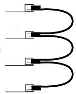
The Expansion Cable (pictured below) has eight 20 AWG wires pre-connected to the lower row (even pins 4-18) of an expansion terminator. The eight wires connect to the upper row (odd pins 3-17) of the next-lower 34934C-001 in the mainframe.
