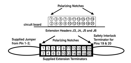
You must fabricate custom cabling to make row signal connections to the central 16 pins (3-18) of these headers, using the pin assignments below. The supplied blue terminators accommodate 22 AWG coated wire, fitted to "crimp-to-wire" contacts with latch tabs.
