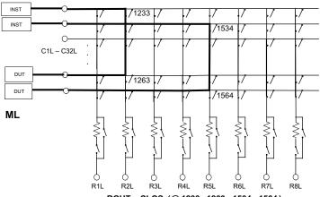
ROUT: CLOS (@ 1233, 1263, 1534, 1564) Closes: row R2L @ columns C1L and C33L row R5L @ columns C2L and C34L
