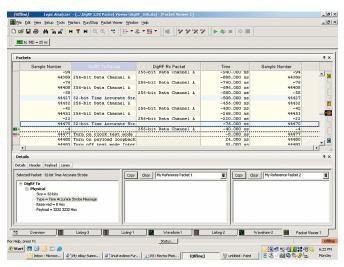
The N4850A probe lets you quickly analyze and debug DigRF v3 control and raw  $\mbox{IQ}$  data at the packet level.
