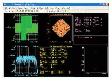
The N4850A probe lets you rapidly work through scenarios. Use the 89600 VSA software running directly on the logic analyzer to quickly identify RF signal problems and fine tune your DSP algorithm.
