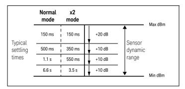
Figure 1-1 8480 Series settling time with auto-filter
