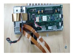
Figure 6-10 Remove the front panel
