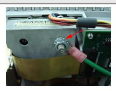
Figure 6-7 Remove the EMI earth wires
