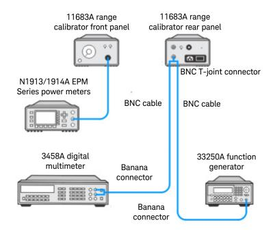
Figure 2-7 Absolute accuracy test setup
