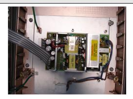
Figure 6-17 PSU cable routing
