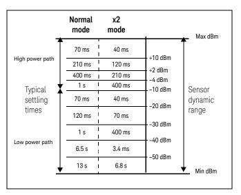
Figure 1-3 E9300 Series settling time with auto-filter
