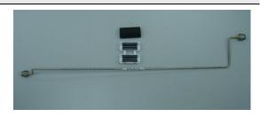
Figure 6-19 Separate the two halves of the ferrite
