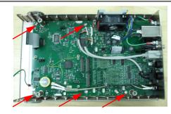
Figure 6-12 Remove the main board
