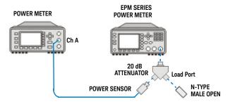
Figure 2-3 Output SWR test setup-open connection diagram
