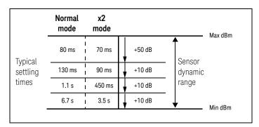
Figure 1-2 E441x Series settling time with auto-filter
