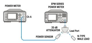
Figure 2-4 Output SWR test setup-load connection diagram
