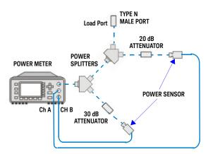
Figure 2-2 System calibration connection diagram
