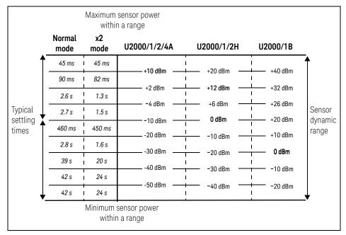
Figure 1-5 U2000 Series settling time with auto-filter
