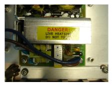
Figure 6-5 Remove the PSU
