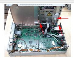
Figure 6-3 Remove the top clamshell
