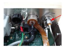
Figure 6-9 Disconnect the semi-rigid cable
