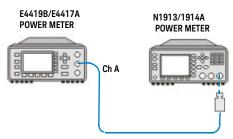
Figure 2-1 1 mW power reference level test setup connection diagram
