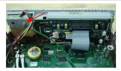
Figure 6-8 Disconnect the front panel cable
