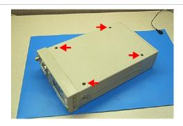
Figure 6-2 Separate the clamshells
