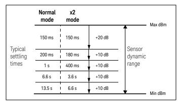
Figure 1-4 N8480 Series settling time with auto-filter
