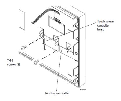
To remove and replace the front panel bracket assembly
