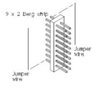
d Solder two resistors to the pin strip, one at each end between the end pins.
