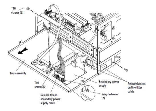
To remove and replace the PCI or display board
