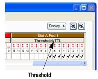
c Verify that the activity indicators (the red arrows) show activity on all 16 channels that are connected to the pulse generator.
