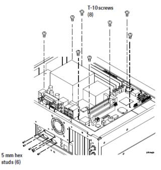
5 Reverse this procedure to install the motherboard.
