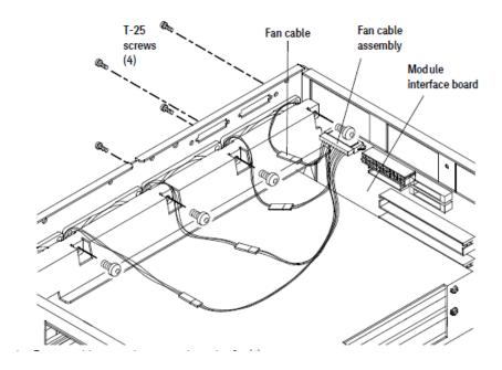
4 Reverse this procedure to replace the fan(s).
