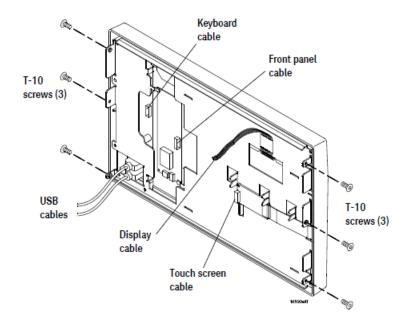
To remove and replace the backlight inverter board
