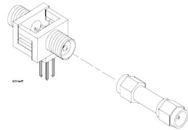
b Attach a 50 ohm terminator to the other end of just one of the SMA/Flying Lead test connectors.
