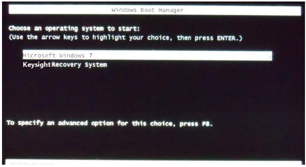
2 After a few seconds, Logic Analyzer automatically starts with the option selected in the Windows Boot Manager. Select the **Keysight Recovery system** option in the Windows Boot Manager screen using the arrow keys and then press Enter.
