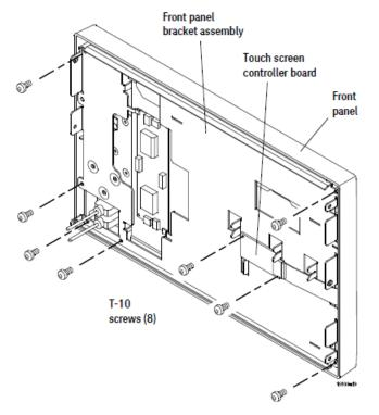
5 Reverse this procedure to replace the front panel bracket assembly.
