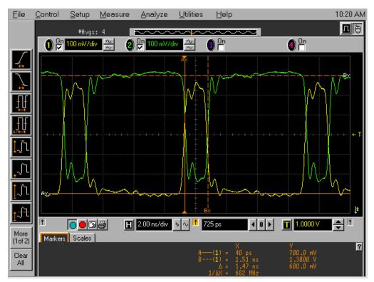
4 Observe the waveforms on the oscilloscope display. If they are not centered within the "Ay" and "By" markers, adjust the 81134A pulse generator's Channel 2 OFFSET until the waveforms are centered as close as possible. (The resolution of the 81134A OFFSET setting is 10 mV.)
