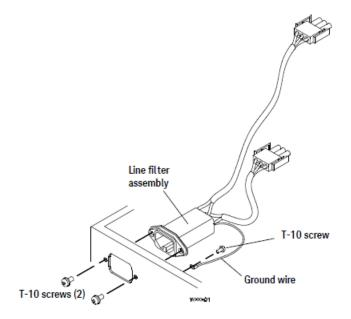
3 Reverse this procedure to replace the power line filter assembly.
