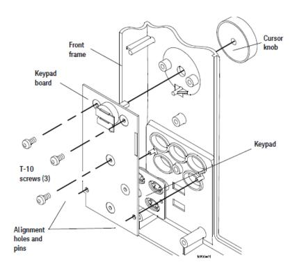
5 Reverse this procedure to install the keypad and keypad board. Note the alignment pins on the frame and the holes in the board.
