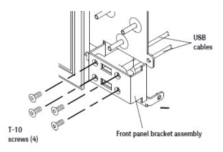
3 Reverse this procedure to replace the USB cables.
