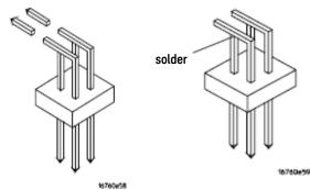
d Using a very small amount of solder, tack each inner lead to each outer lead at the point where they are touching.
