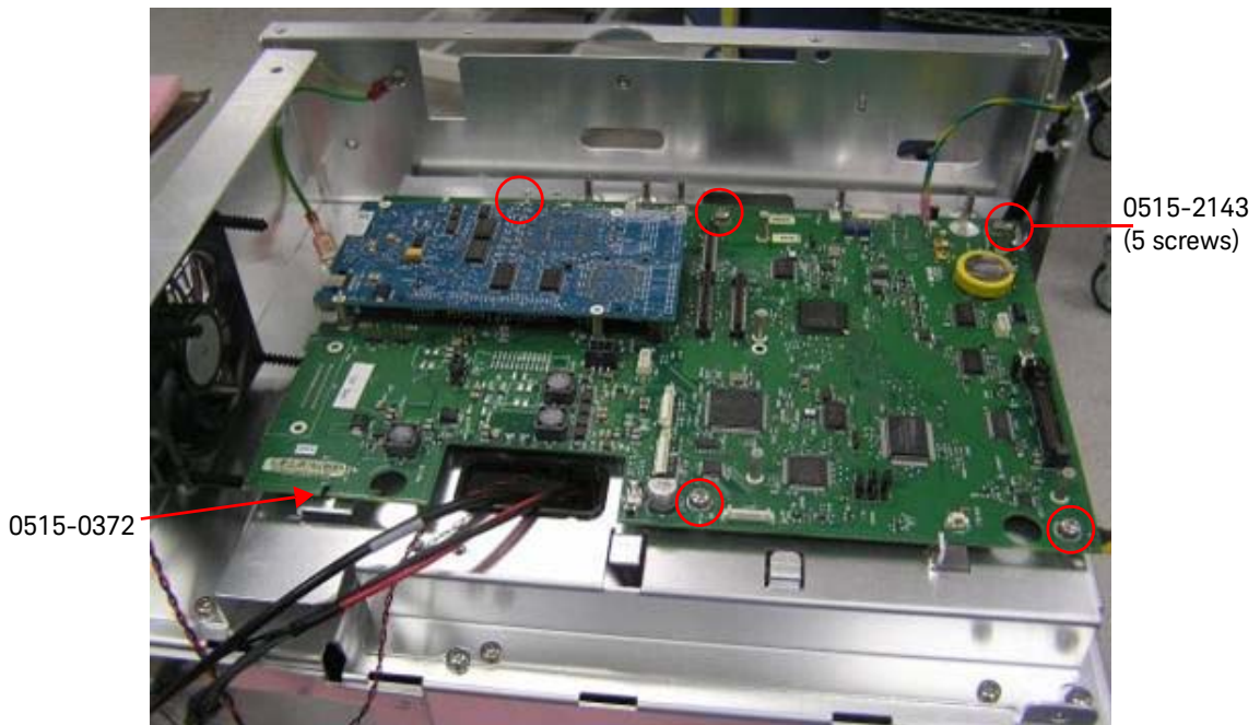
Figure 4-46 Remove the mainboard
