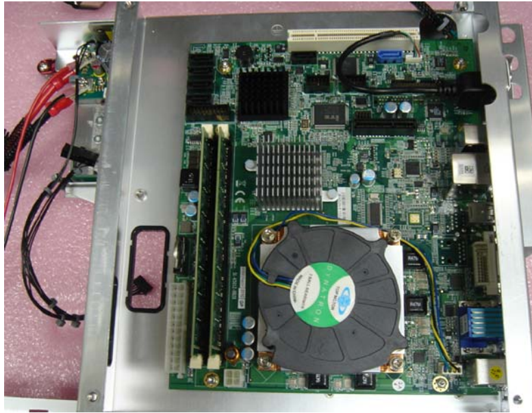
Figure 4-62 Power supply deck assembly with the power supply module and PC motherboard
