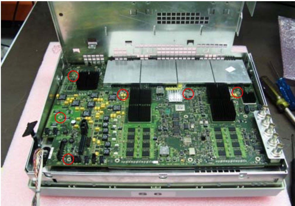
Figure 4-70 Uninstall all the connectors
