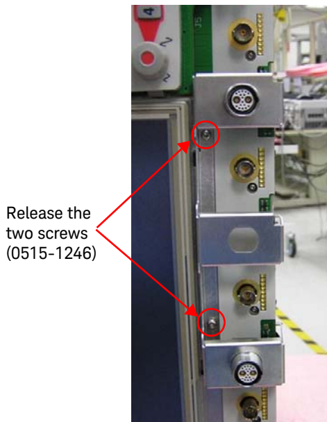
Figure 4-16 Unslot the N-type connector and release the two screws
