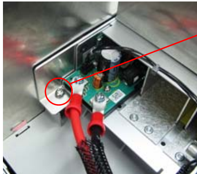
Figure 4-60 Uninstall the power supply deck assembly
