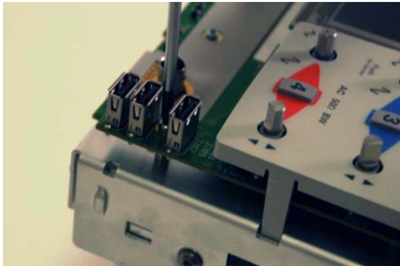
Figure 4-19 Remove the screw near the front panel USB ports
