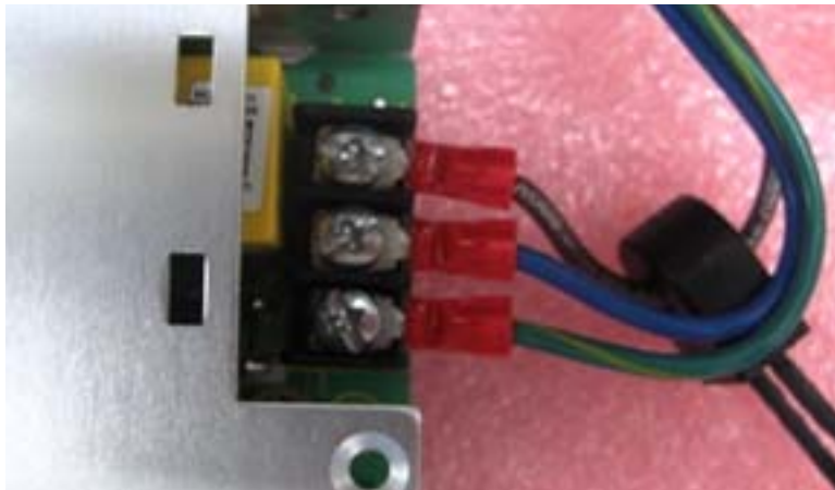
Figure 4-64 Remove the power cables connected to the power supply module
