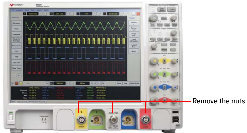
Figure 4-12 Remove the nuts at the sensor connector and the N-type connector
