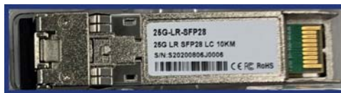
Figure 18 SFP28 module (top view)
