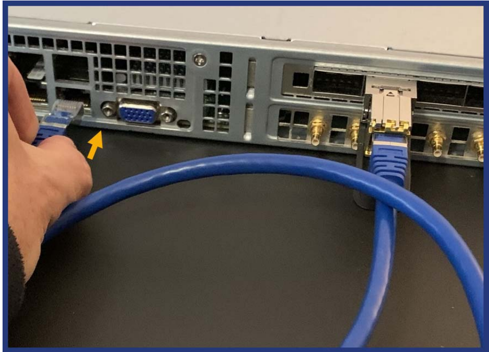
Figure 39 Inserting the Cat-5 cable to the secondary Ethernet port
