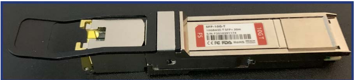
Figure 36 Inserting a Copper SFP module into a QSFP28 to SFP28 adapter
