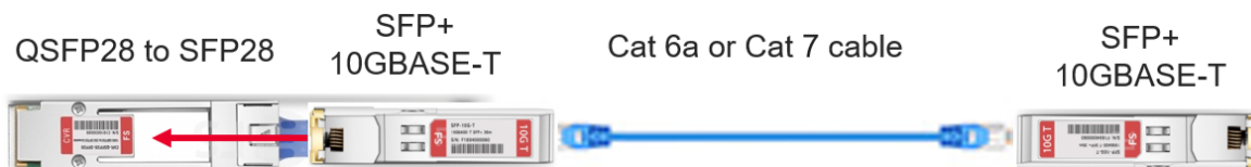
Figure 8 QSFP28 to SFP28 adapter with 10GBASE-T Copper
