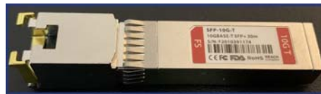
Figure 19 Copper SFP module (top view)
