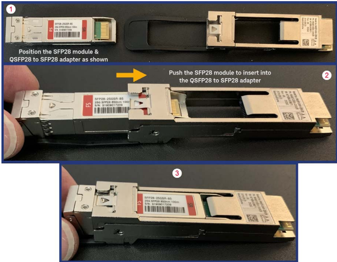
Figure 29 Inserting SFP28 module to a QSFP28 to SFP28 adapter
