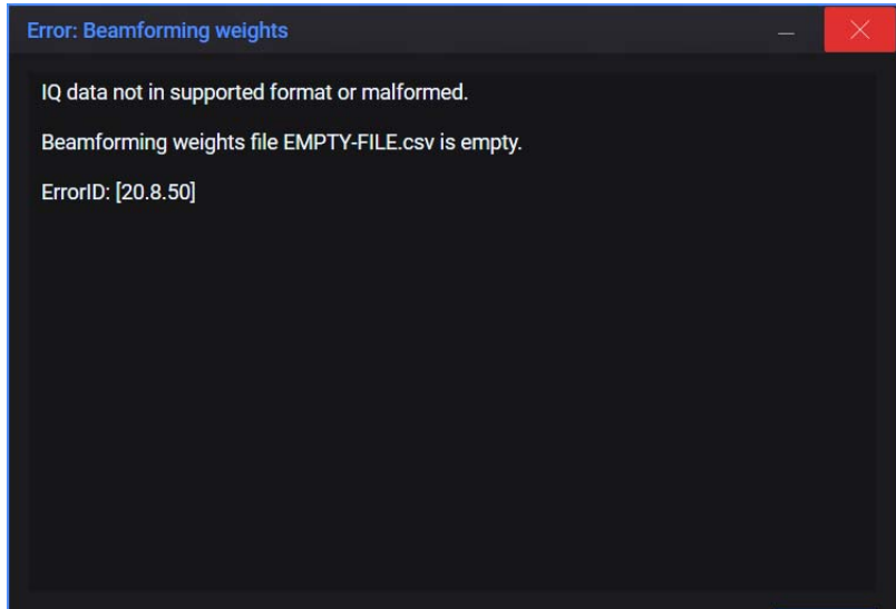
Figure 308 Error when loading CSV file that is empty
