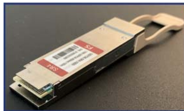
Figure 17 QSFP28 module (lateral view)
