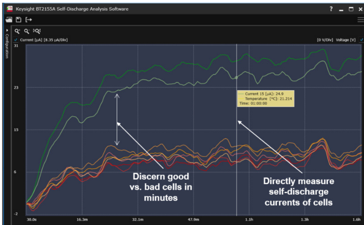
Figure 4. Self-discharge current measurements of multiple Li-ion cells using the Keysight BT2152B
