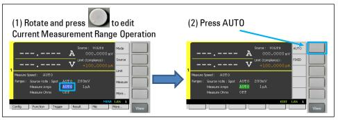
Step 2. Rotate and press to edit the current minimum measurement range, and then select to set it to 10 nA.
