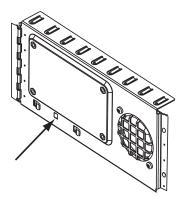
**2** Remove the safety shield. Using a T20 Torx, remove the four screws holding the power supply printed circuit board to the sheet metal.
