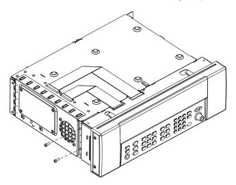
2 Swing the module out and disengage it from the sheet metal at the back.
