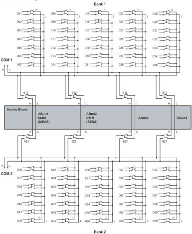
For the 34922A, relay part numbers are given on page 136 and the component locator is shown on page 145. The table on the next page shows the relationship of channel numbers to relay numbers.
