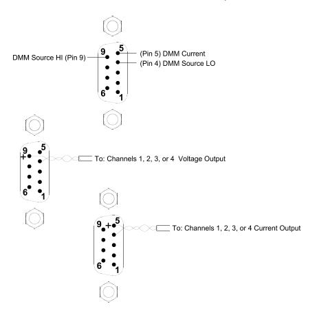
Analog Output Verification Test This procedure is used to check the calibration of the analog outputs on the 34951A 4-channel DAC Module. Verification checks are performed only for those output values with unique calibration constants.
