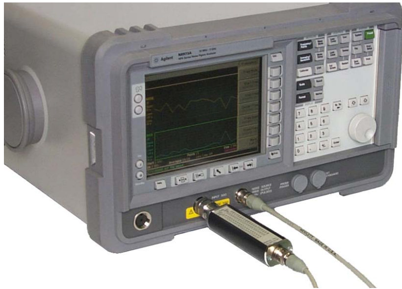
Figure 1-1 NFA with a Normal Noise Source connected
