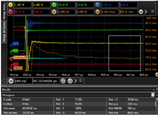
Figure 3: Turn-on switching waveform of a 650 V rating GaN E-HEMT obtained by the newly developed GaN test board with a clamped circuit.
