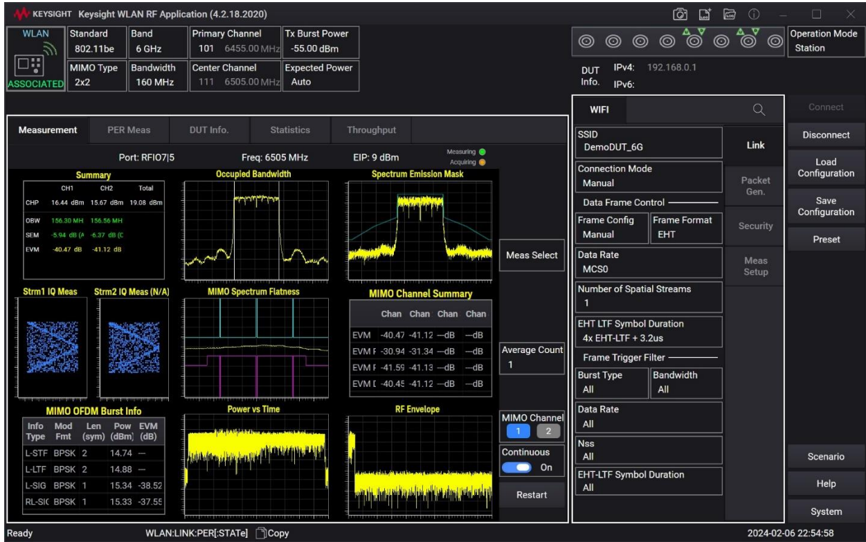
Figure 1 below shows the Keysight S8714A UXM 5G RF application running 802.11be (Wi-Fi 7) measurements.
