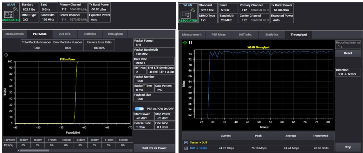
Figure 1. Keysight S8714A UXM 5G RF application running 802.11be (Wi-Fi 7) measurements for RF analysis.
