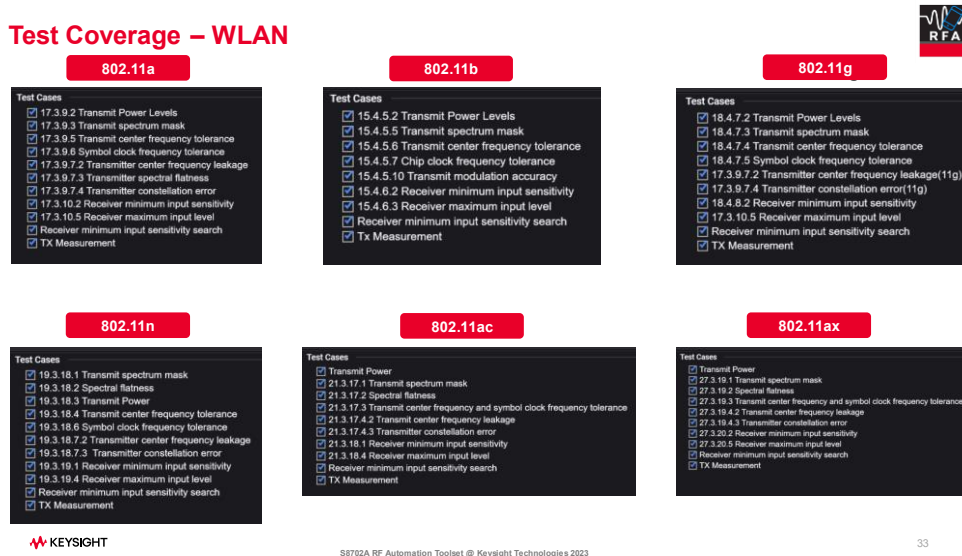
Figure 3. Wi-Fi test cases coverage for each technology in S8702A RF Automation Toolset
