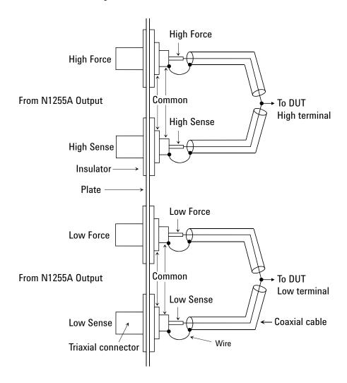
The High Force/High Sense/Low Force/Low Sense lines should be connected to the DUT as shown in Figure 3-9. Wiring shown in Figure 3-14 Cable and Probing needle can be used. To simplify the connections, omit the wiring of the Common.
