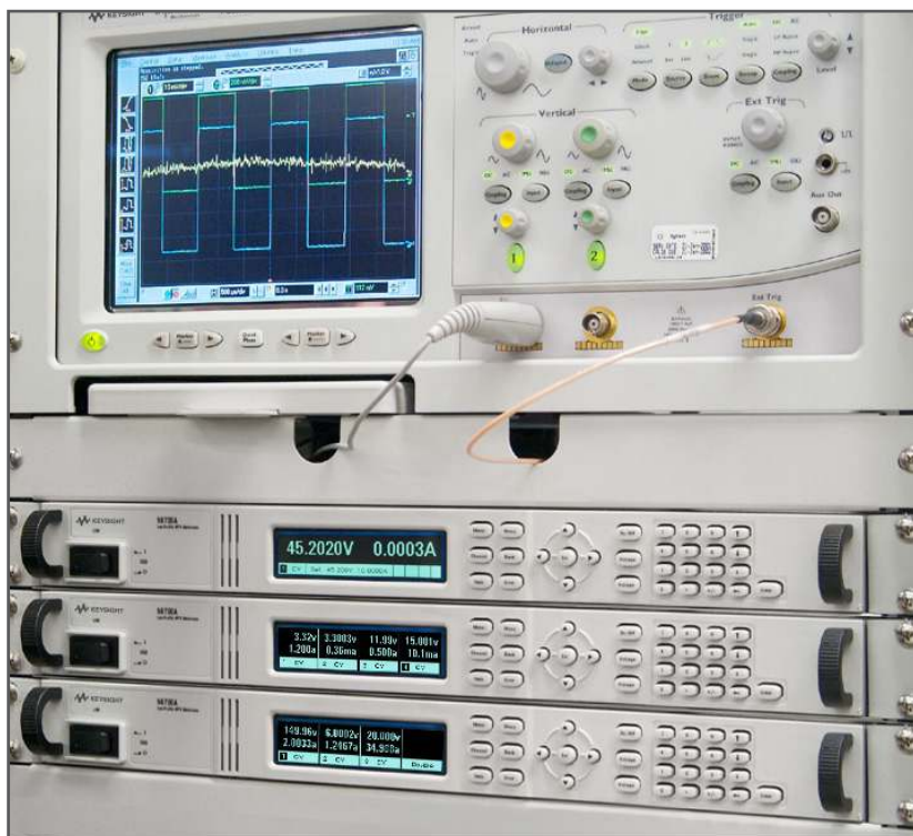
Figure 1: Three low-profile (1U) multiple-output modular power systems are shown installed in a test rack. Each of the three power systems can hold up to four power supply outputs, each with its own voltage and current readback.
