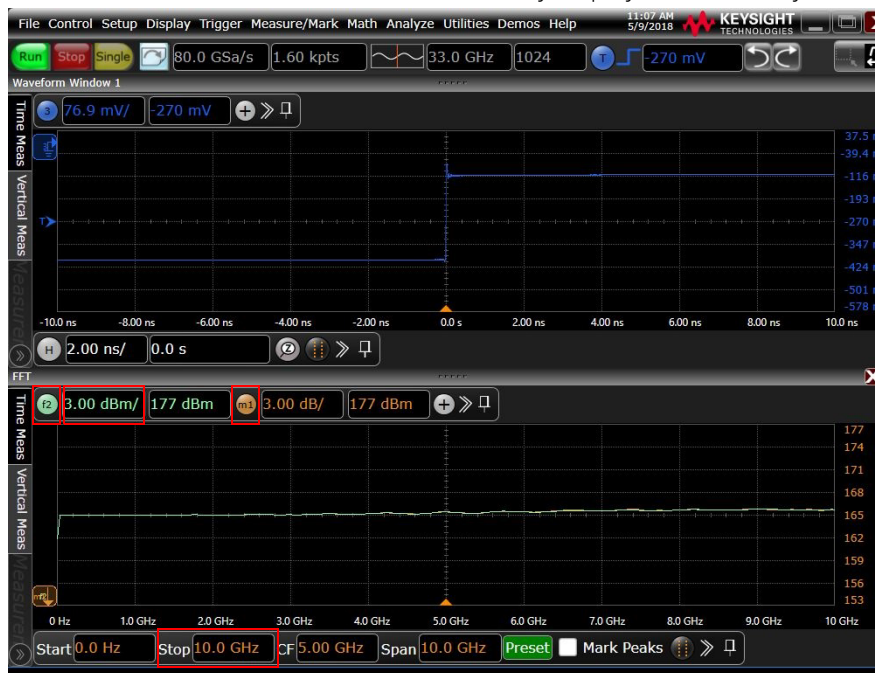
Figure 30 Frequency response of the Cal Out step through the attached coax cable
