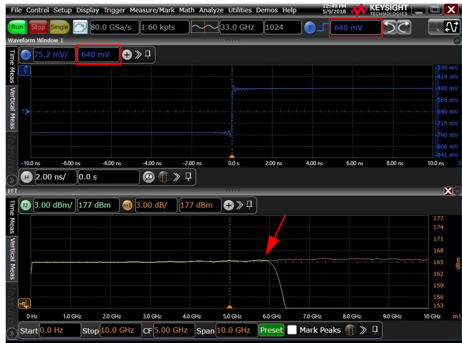
Figure 32 Frequency response of the N7024A probe
