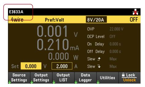
Figure 6. Enable E3633A/E3634A mode on the E36231A and E36232A
