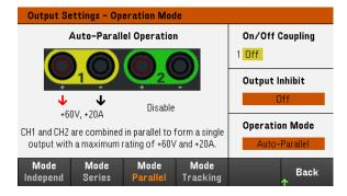
Figure 3. Auto-series and parallel operation together doubles the output voltage/current
