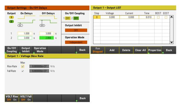
Figure 8. Output sequencing and output LIST mode, with slew rate setting
